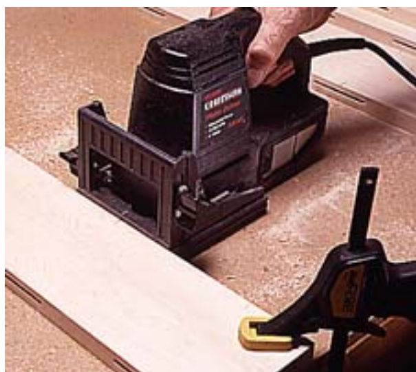
1--Joint the edges of the boards for the tabletop and cut the slots in them to receive the joining plates.
