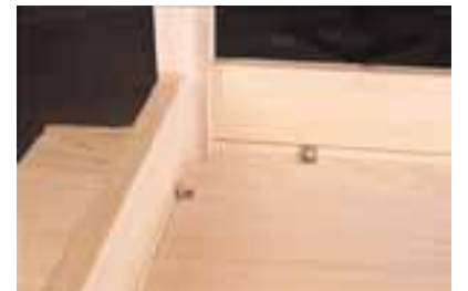
These table top fasteners are cheap ($1.99 for a pack of eight) and sturdy. Simply place the clip end into the kerf in your apron and screw the other end to your table top.
