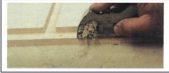
Cleaning up a rabbet joint with a shoulder plane
