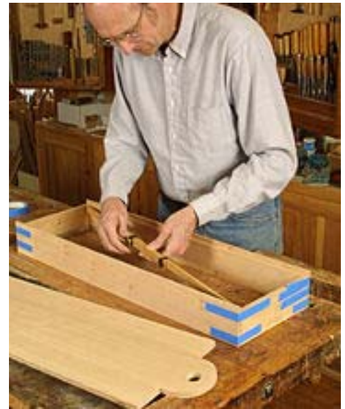
The false top and false bottom are simply butt-joined and glued to the sides. The actual top and bottom will reinforce this joint. Before the glue sets, check to make sure the case is level and square.
