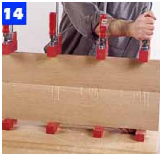
Begin assembly of the top by joining only two boards. After the glue cures, add one board at a time to reach full width.
