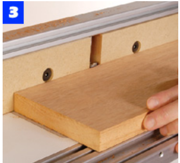
Shim the outfeed fence of a router table so it's aligned with the bit, and use your table to joint the stock edges.
