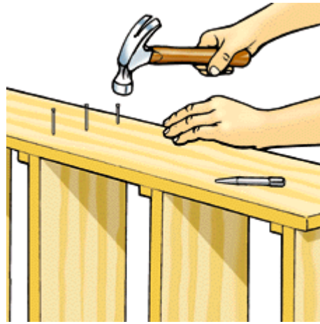
Fig. 7 Secure one side to the shelves with glue and 6d finishing nails. Then flip the assembly over and attach the other side. Set all nails.
