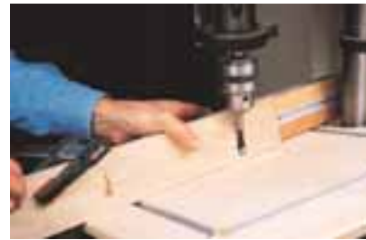
Another view of the drill-press table. Here I'm cutting pocket holes in a table apron.
