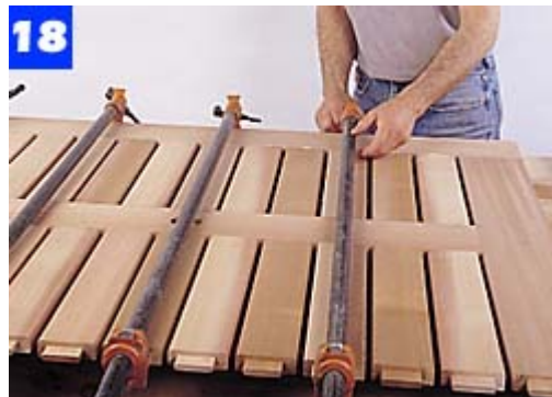
Clamp one stile at each end of the top subassembly. Space clamps evenly and at the center of a tenon.
