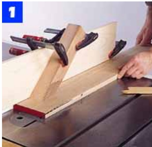
With a featherboard holding the stock against the table, rip a 45° bevel on both edges of each leg face board.
