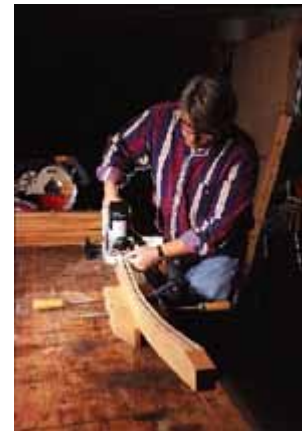
Holding the arched top rail steady was the most difficult part of routing the top groove for the slats. Remember to make the cut in two passes on each side. In this photo you can see that the rail hasn't been cut for length yet, allowing extra support for the router at the beginning and end of the cut.
