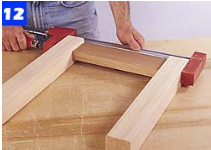
Glue and clamp together a pair of bench legs and one short apron. Make two of these subassemblies.
