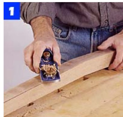
After sawing the rear leg shape, use a sharp plane to remove saw marks and trim the leg to exact size.
