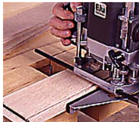
14--Use the same dovetail bit in a router table to cut both sides of the dovetails on the ends of each drawer side.
