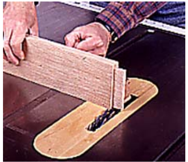
3--Use a dado blade in a table saw to cut the rail tenons. First cut the cheeks, then readjust the saw to cut the shoulders.
