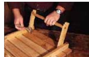
Last, but not least, bolt the table legs in place to the table battens. Note the notches on the ends of the legs which drop into the previously cut notches to stabilize the table.
