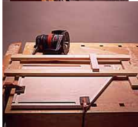
4--Cut grooves and dados in the end panels with a router. Then tack nail a block across the rails to stop the cut.
