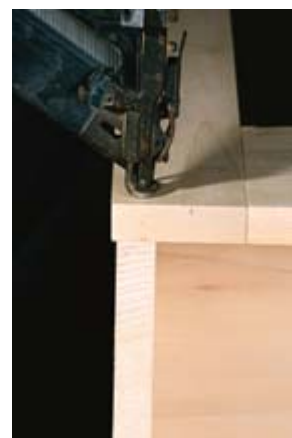
I'm not perfect, and neither are you. If your face frame is exactly the width of your case, it's going to be difficult to fasten it square. Make life easier by ripping your stiles \frac{1}{16} " oversize in width. After you nail and glue the face frame to the case, use a flush-trimming bit in your router to trim the face frame flush with the side of the cabinet's case.
