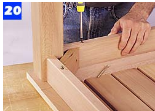
Attach the tabletop to the base with several screws. Drive each screw into its matching counterbored hole in the apron.
