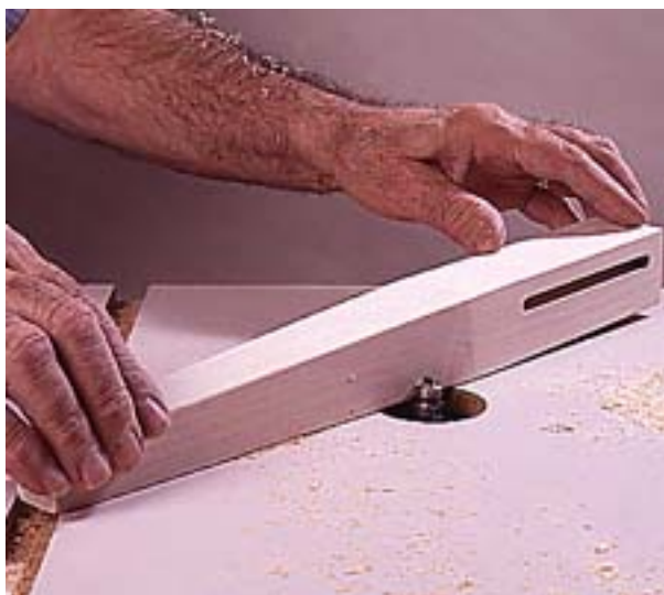
6--Round the bottom of the leg corners on the router table. Don't round the top of the leg where it abuts the apron.
