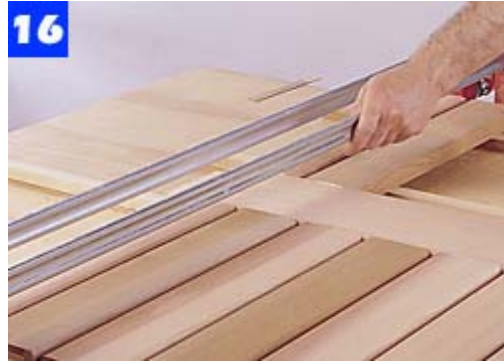
A second set of slats is glued and clamped to the center rail. Again, use one clamp in the center of each slat.
