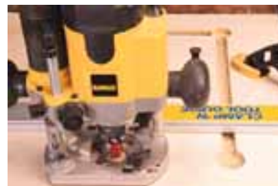
ROUT THE GROOVE The grooves for the T-slot track allow the fence to be used left-to-right and front-to-back on the table to take advantage of the built-in tilting feature of the existing table.
