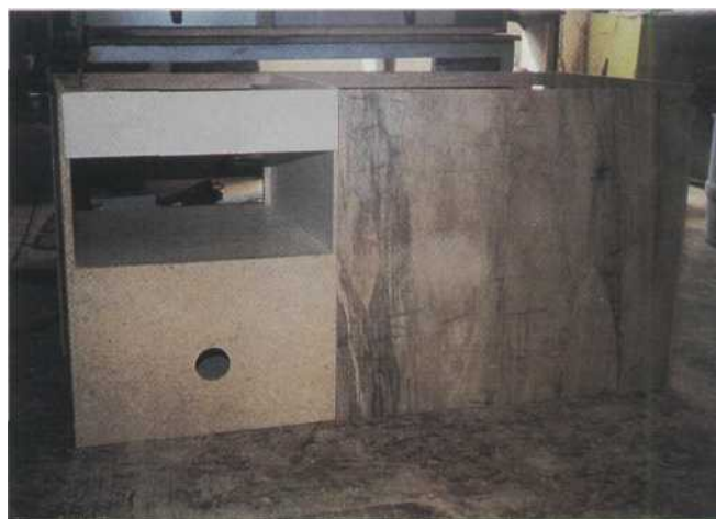
3 The three backs in the desk unit shown in place. Notice the wire chase hole for the printer drawer.
