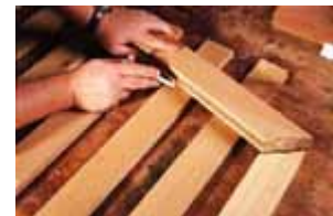
With the miters cut on the top rail and back stiles, space the slats and use the top rail to mark the angle and length of each slat, (adding 1").
