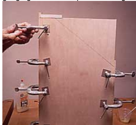
2--Glue and clamp each of the edge bands to the panels. Note that the top edge band of the end panel is just slightly long.
