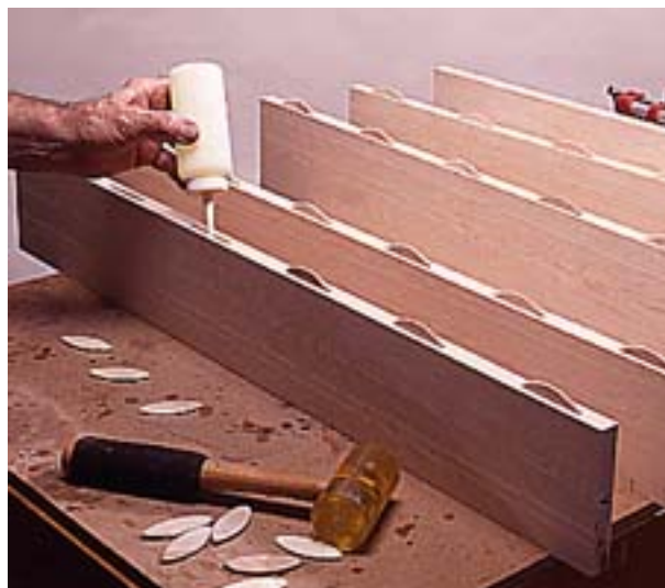
1--Joint the edges of the boards for the tabletop and cut the slots in them to receive the joining plates.
