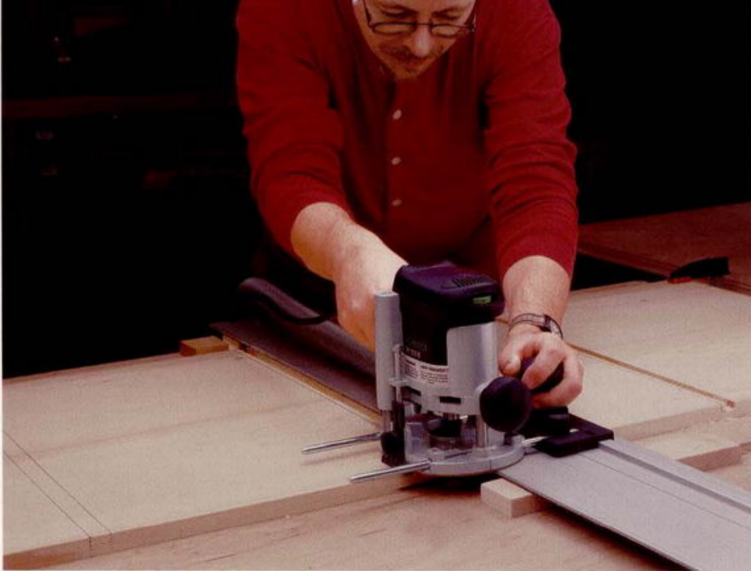
Photo A: Rout the dados for the shelves in the sides with the sides clamped back edge to back edge.
