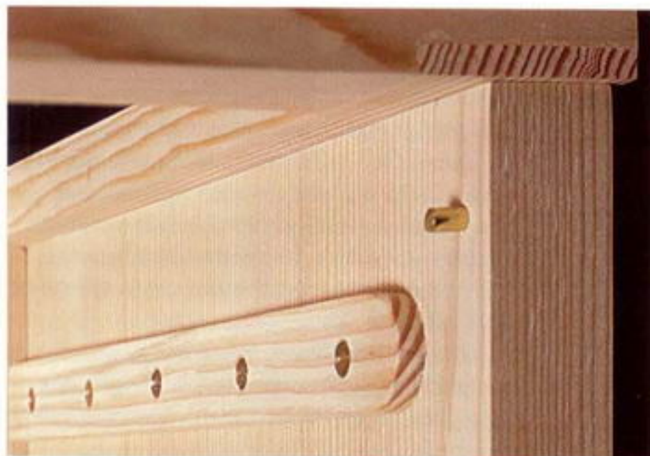
A simple pin and ledger strip are enough to guide and support the door in the open position.
