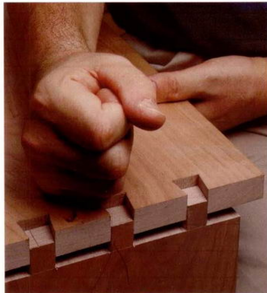
Photo D: You should be able to push or lightly tap a dovetail joint together. Any tighter and it will bind when glue is applied.
