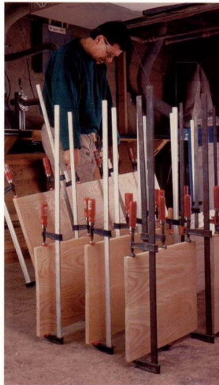
Photo A: The bookcase sides and shelves are wide ( 9\frac{1}{2} in. to 13\frac{1}{2} in.), and have to be glued up from two or more pieces.
