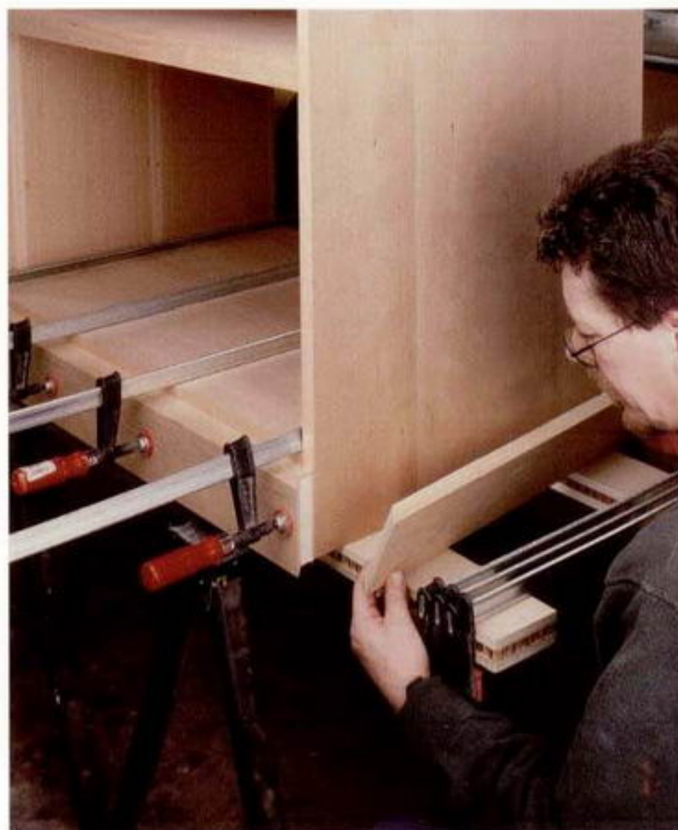
Photo D: Simply glue the three baseboards in place. Add a backing block in front so the base stands proud of the doors the same distance the side pieces stand proud of the sides.
