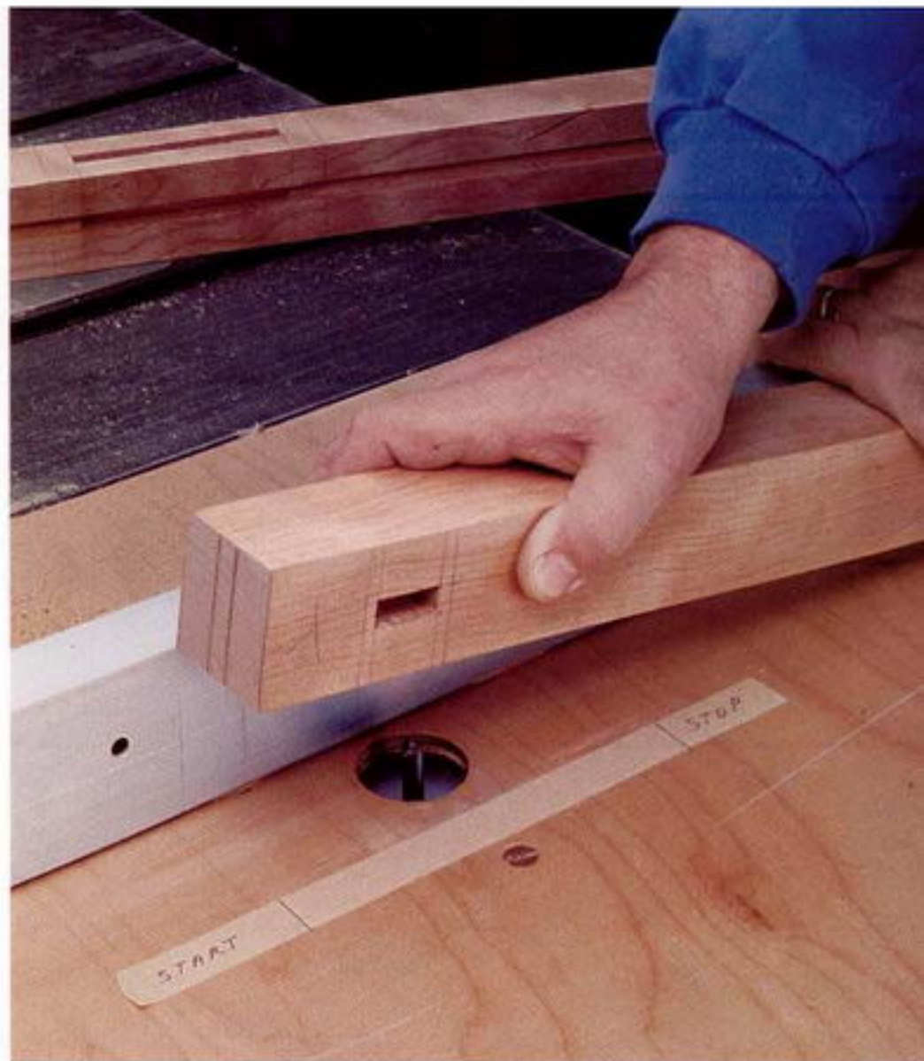
Photo B: Cut the panel grooves in the posts on a router table. Start and stop the cuts from inside the mortises where the bit can't catch as you lower the post down or lift it off.
