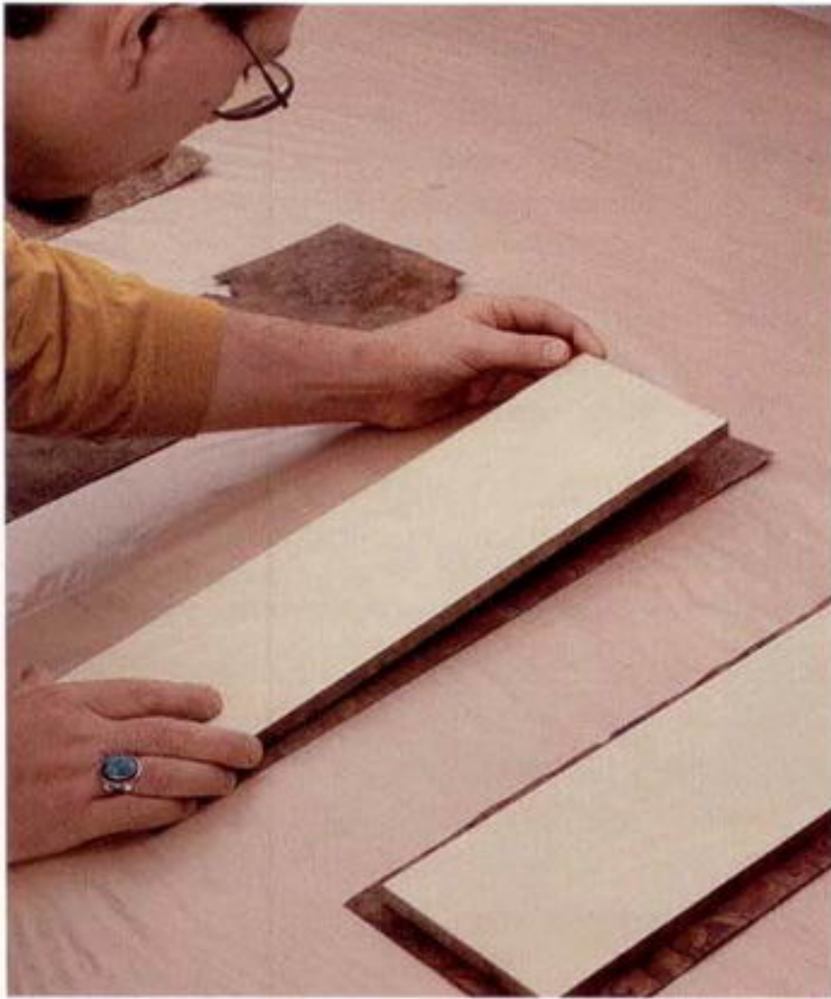
Photos D and E: Vacuum presses make applying veneer to the drawer fronts and side panels a cinch. Just position the pieces on the veneer in the press (left). Lower the membrane top and start the vacuum pump. The bag exerts perfectly even pressure over the parts (right).
