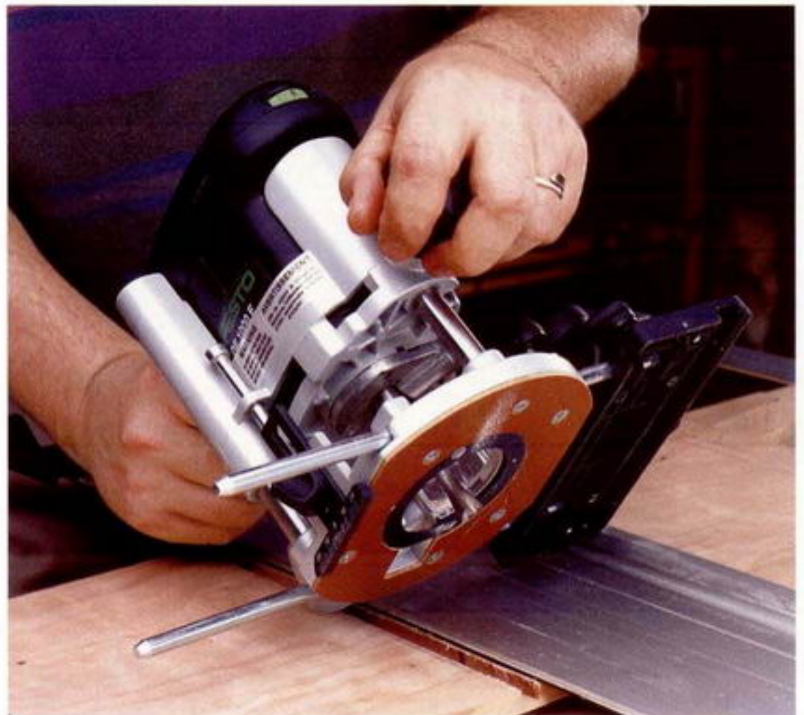
Photo H: The guide rail guides the router accurately through the cut by means of a stop that attaches to the router and precisely fits the guide rail.
