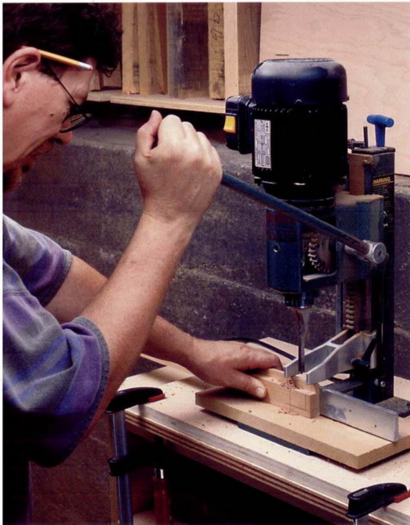
Photo Q: The door frame mortises on the four stiles are cut using a hollow-chisel mortiser.
