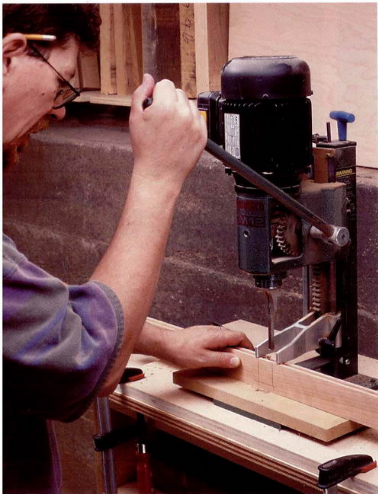
Photo P: The mortises in the rails of the back frame are easily cut on a hollow-chisel mortiser.
