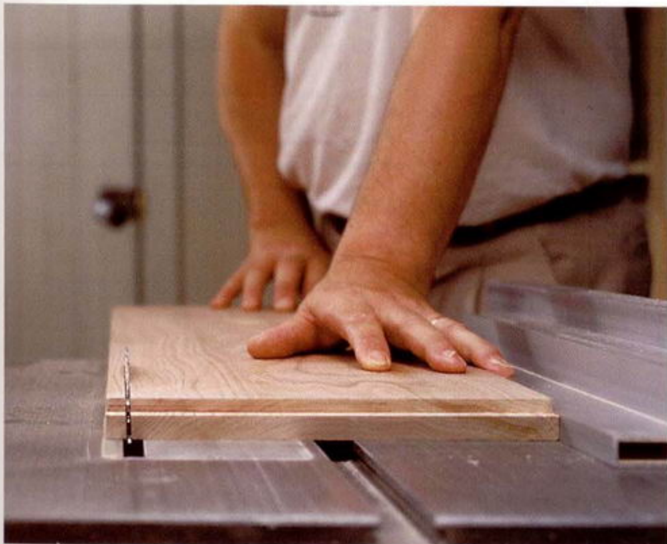
Photo H: Rip the small angle on the front edge of the shelves on the table saw.
