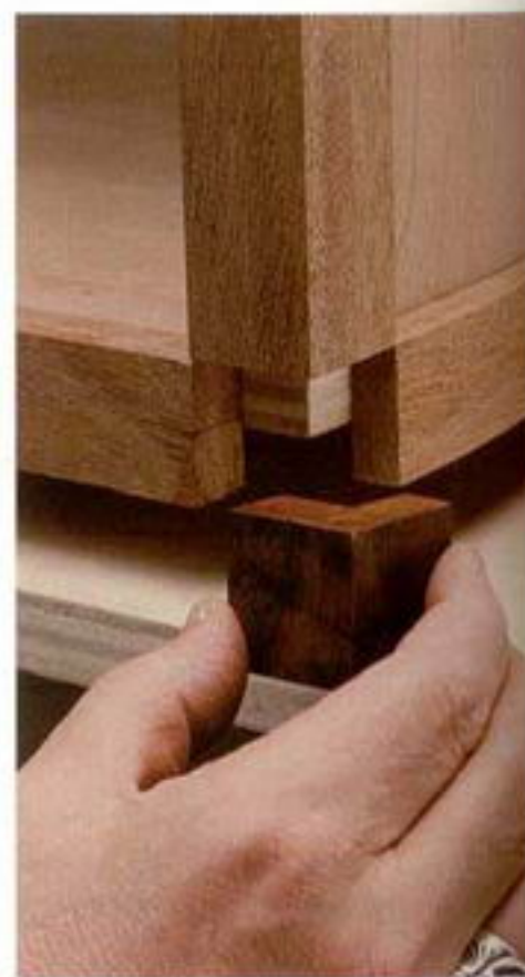
Photo C: Glue the finished corner blocks in place. There's not much glue surface for them to attach to now, but they will be supported later by the feet.
