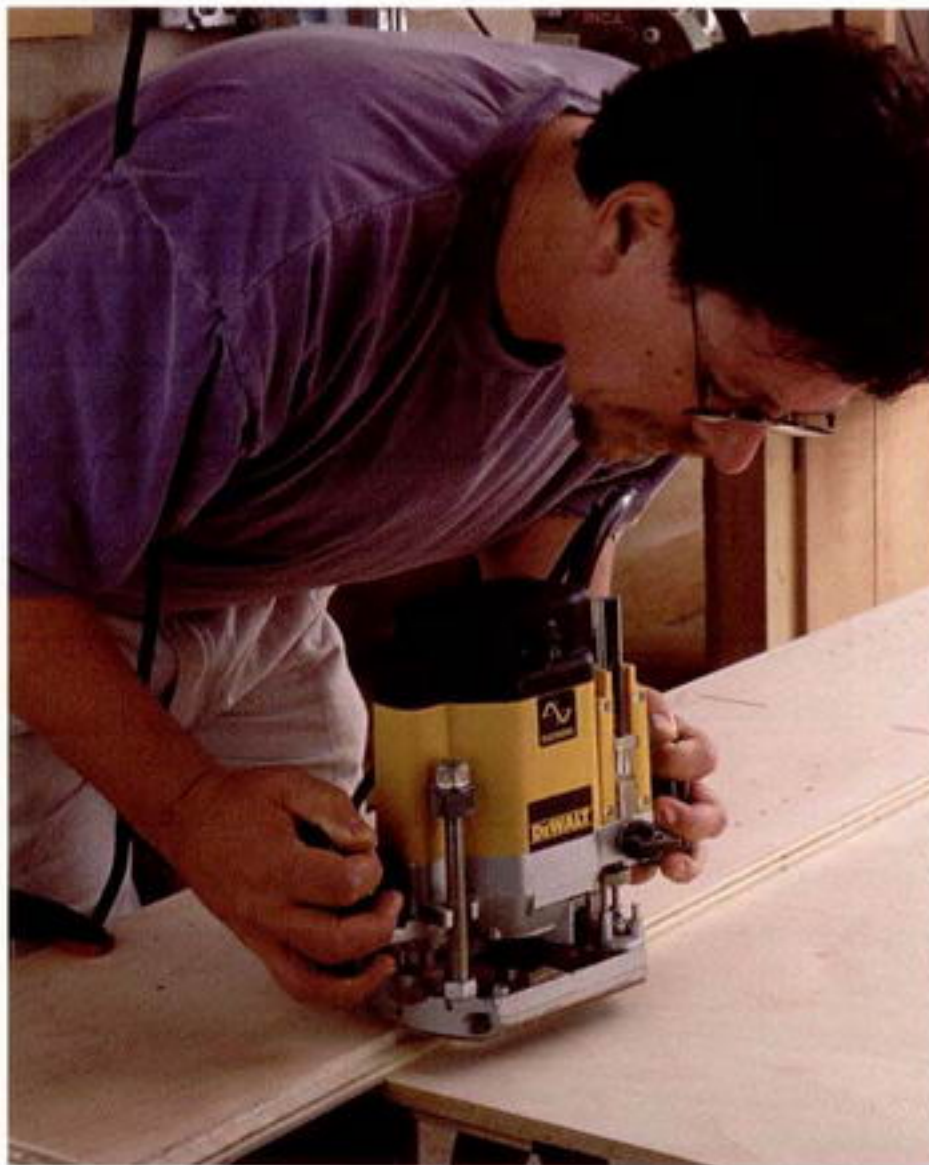
Photo A: Cutting the rabbet in the sides is easy with a router and a ½-in. piloted bit. It's especially useful for the stopped cut on the top edge.
