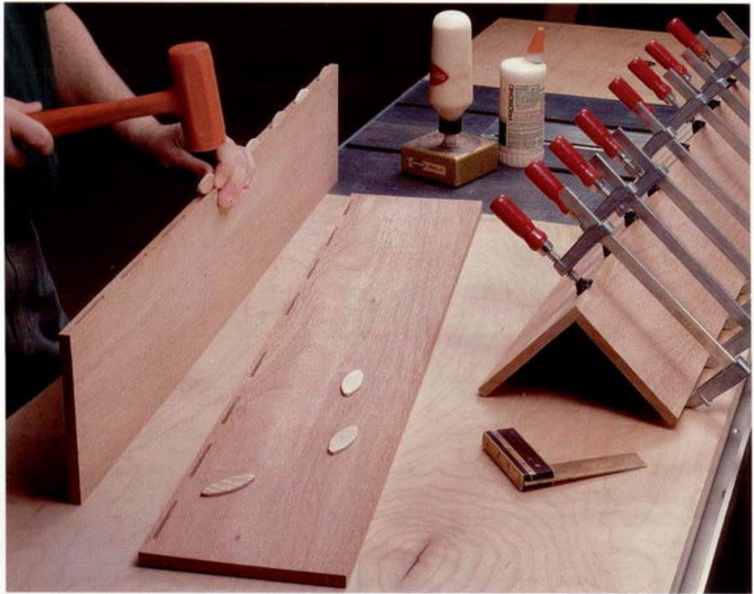
Photo D: Cut biscuit slots in the edges of the narrower pieces and the faces of the wider pieces. When gluing, put a clamp over each biscuit for even pressure.
