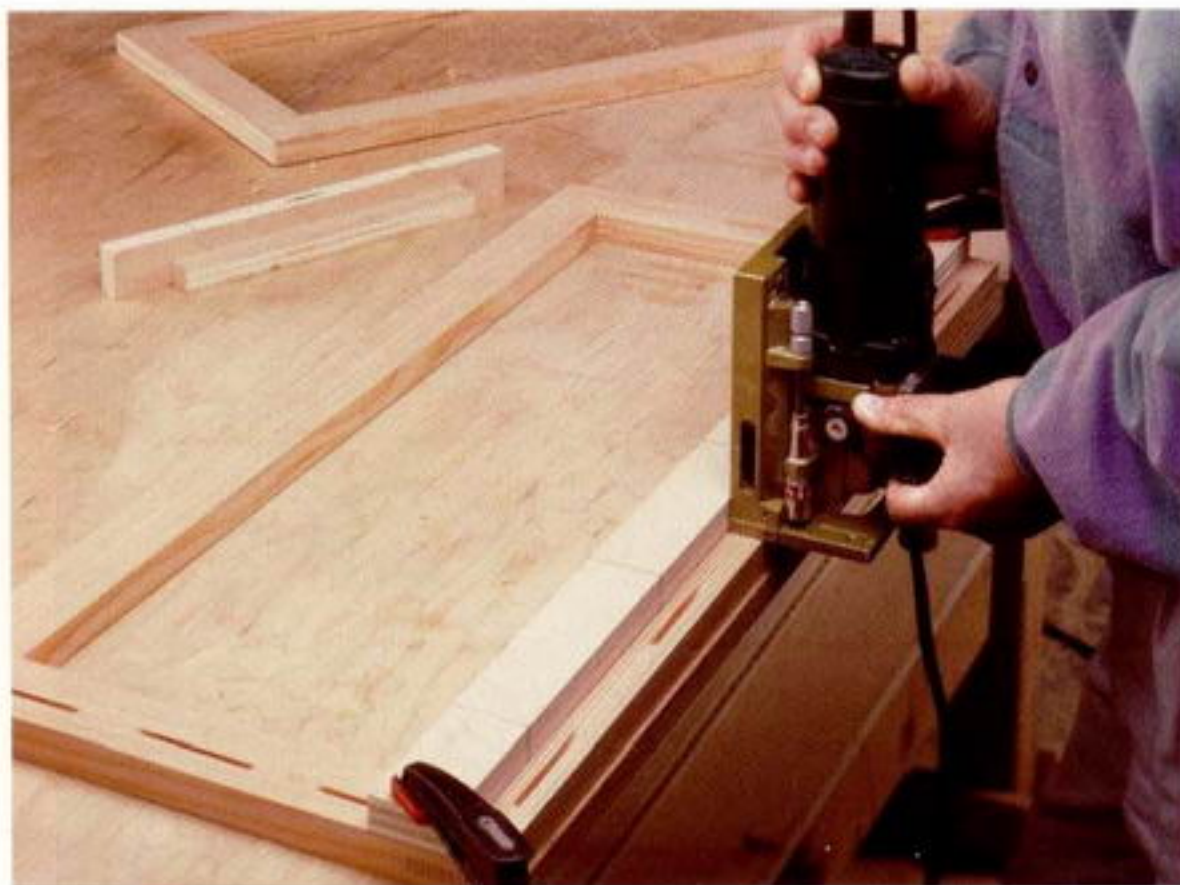
Photo E: Clamp a fence along the line where the side intersects the frame to guide the biscuit joiner.
