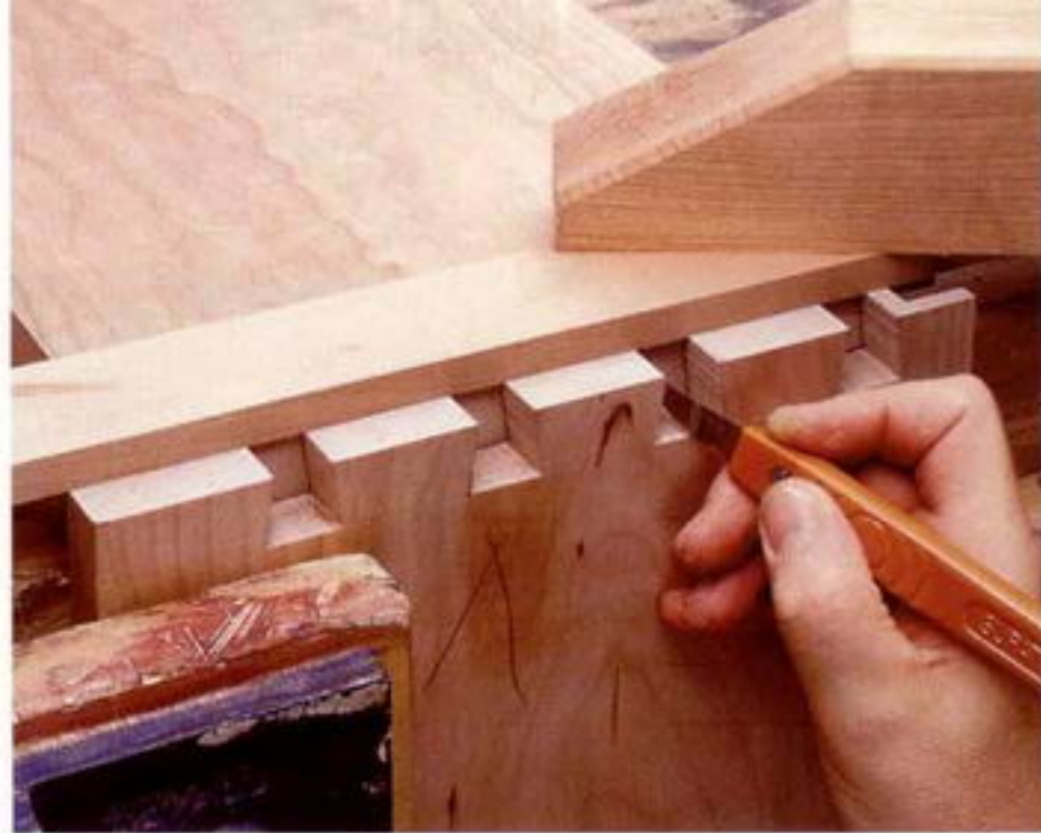
Photo B: Align the top and side the way they will go together and use the cut tails to mark the pin locations. A sharp knife with a point will give you great accuracy.
