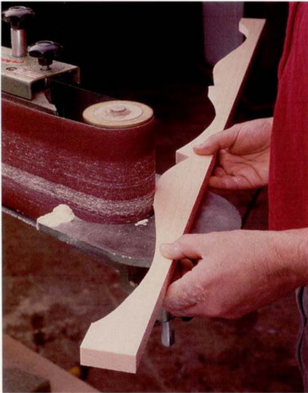
Photo F: A stationary sander does a good job on the larger profiles. Smaller profiles have to be worked with smaller sanders and by hand sanding.
