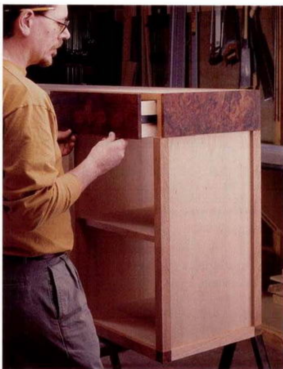
Photo H: Adjust the fit of the drawer front on the drawer or on the glides.
