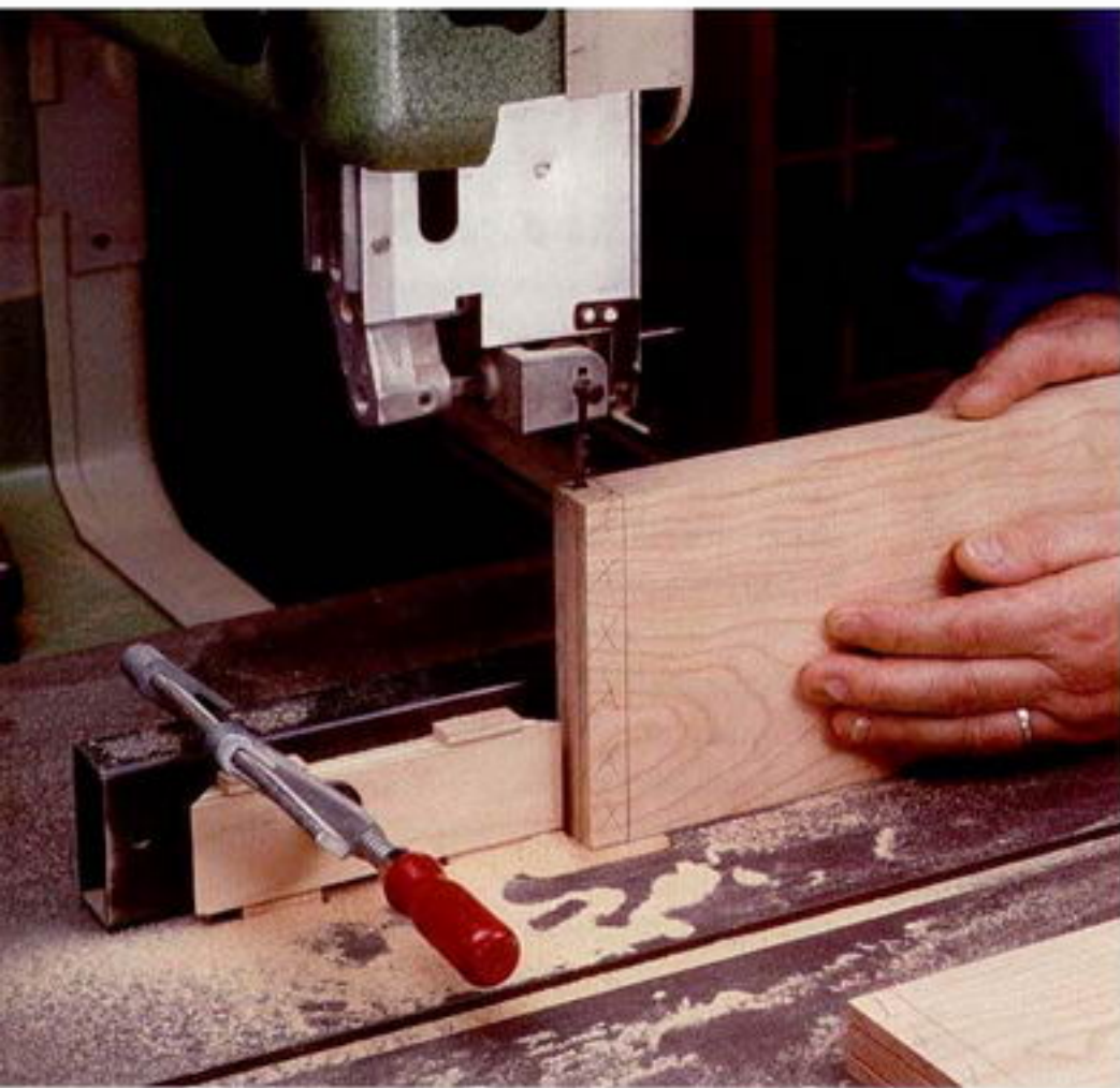
Photo D: Cut the tenon cheeks of the rails and stiles on the bandsaw. Clamp a block to the fence as a depth stop.
