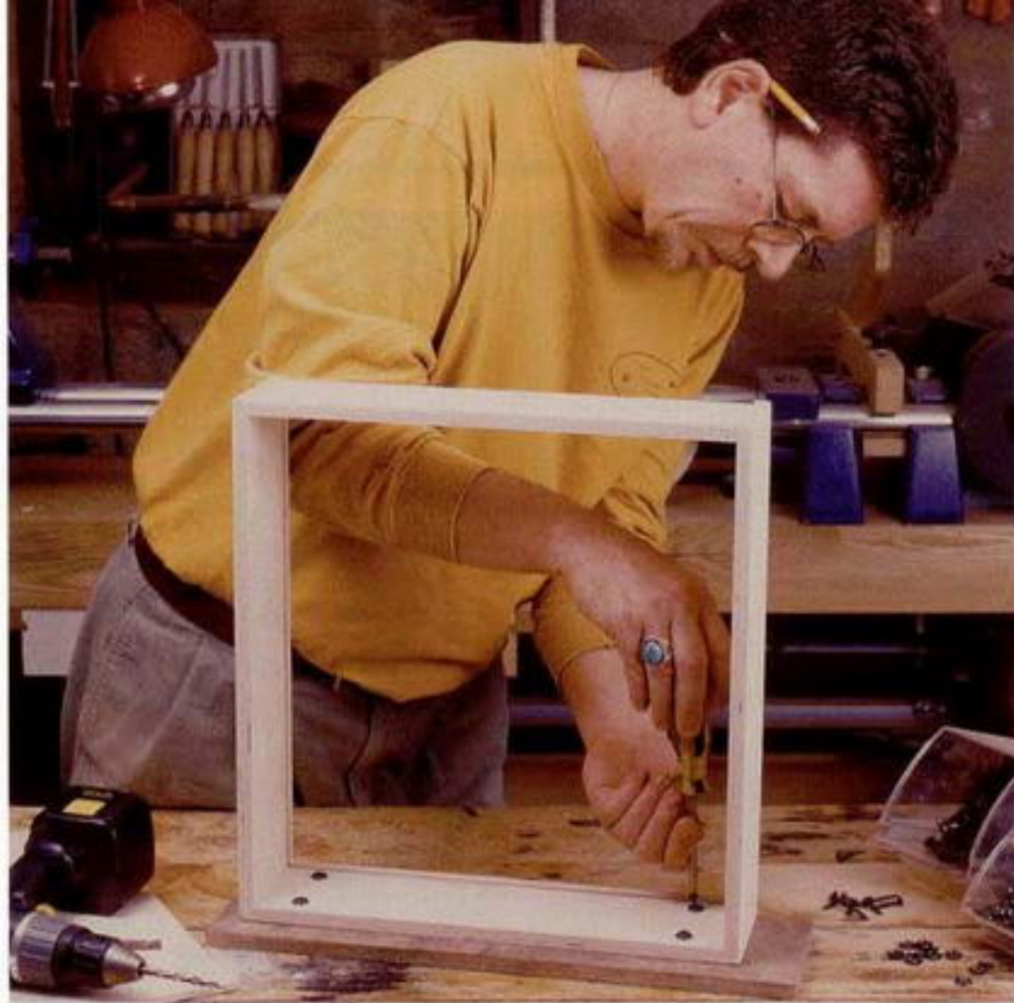
Photo F: Screw the drawer carcass to the drawer front through holes that are slightly larger than necessary. These holes will make it possible to adjust the way the drawer front hangs when installed.
