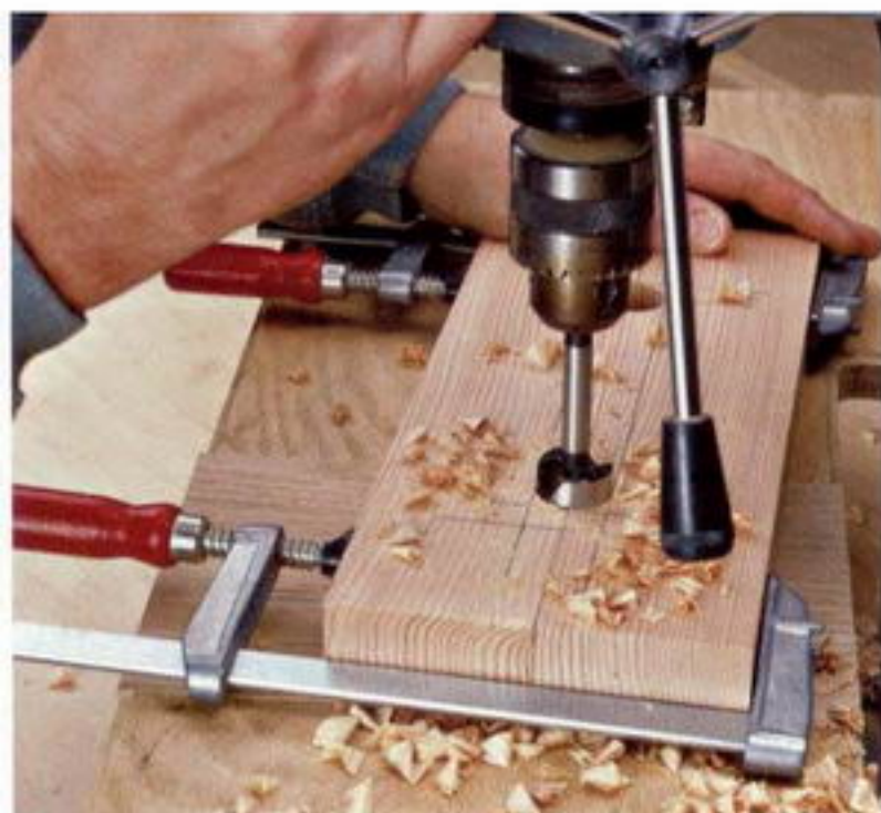
Photo H: Clamp the bottom edges of two base sections and drill a 1-in. hole between them to form the half-round corners at the ends of the cutout.
