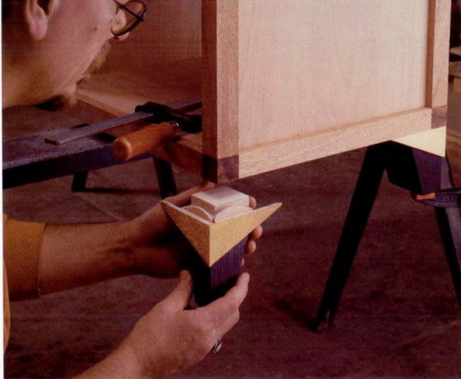
Photo K: The complex foot assembly, with alignment biscuits and spacer block, is simply glued in place.
