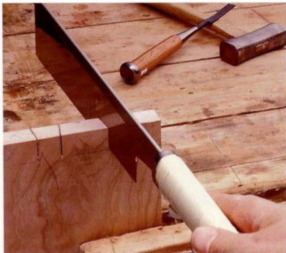
Photo C: Saw the sides of the pins with a fine-toothed backsaw slightly away from the line. A Japanese or Western backsaw will do the job well.
