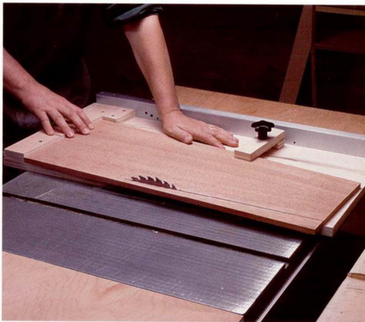
Photo A: A simple taper jig cuts the angle on the side. With the registration block, it also ensures the sides are uniformly wide.
