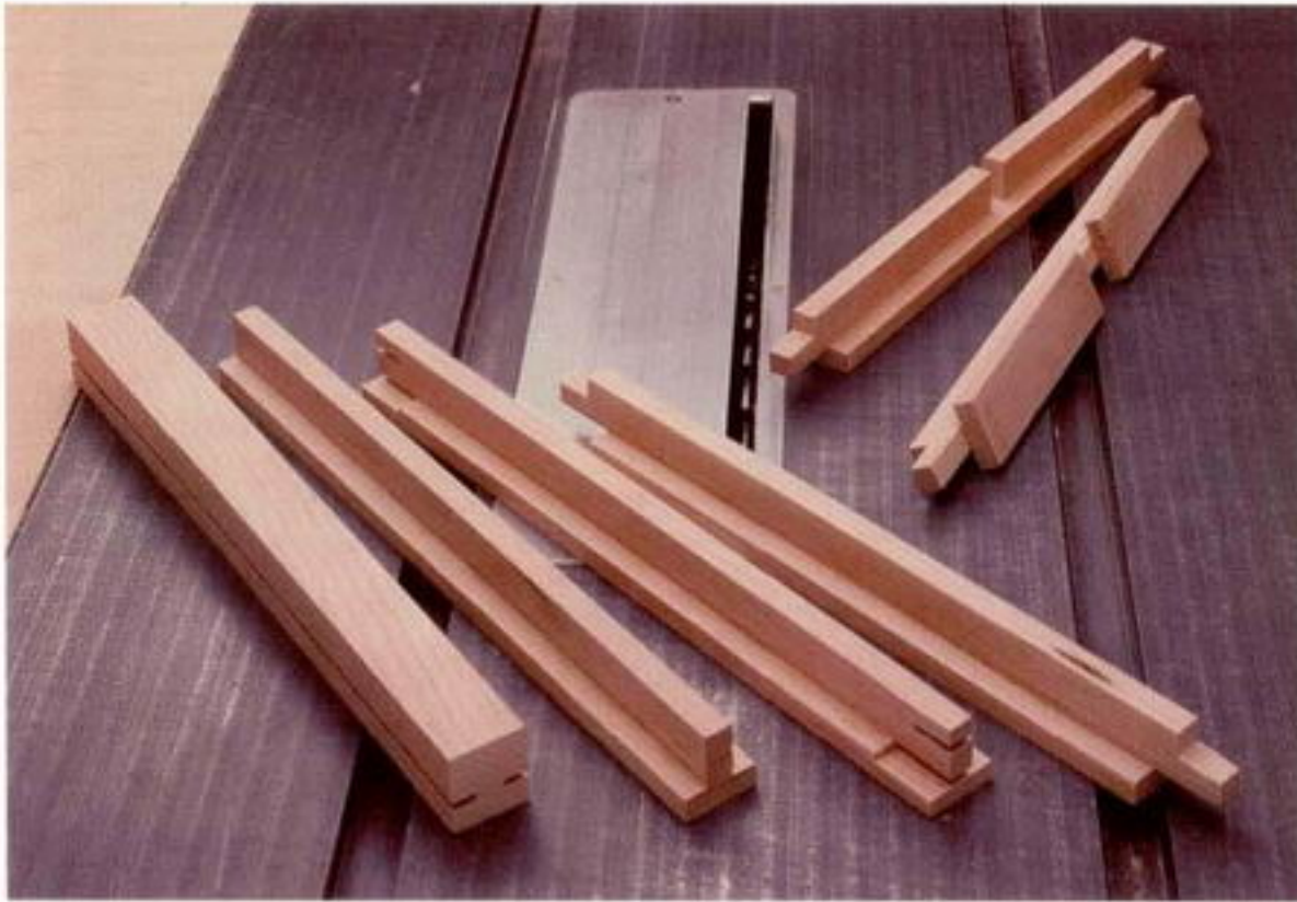
Photo G: The sequence of table-saw cuts in the muntins begins (left to right) with two rips to create the rabbet, two more in a tenoning jig to form the faces of the tenon, two crosscuts to determine the shoulders of the tenon, and several more crosscuts to create the half-lap.
