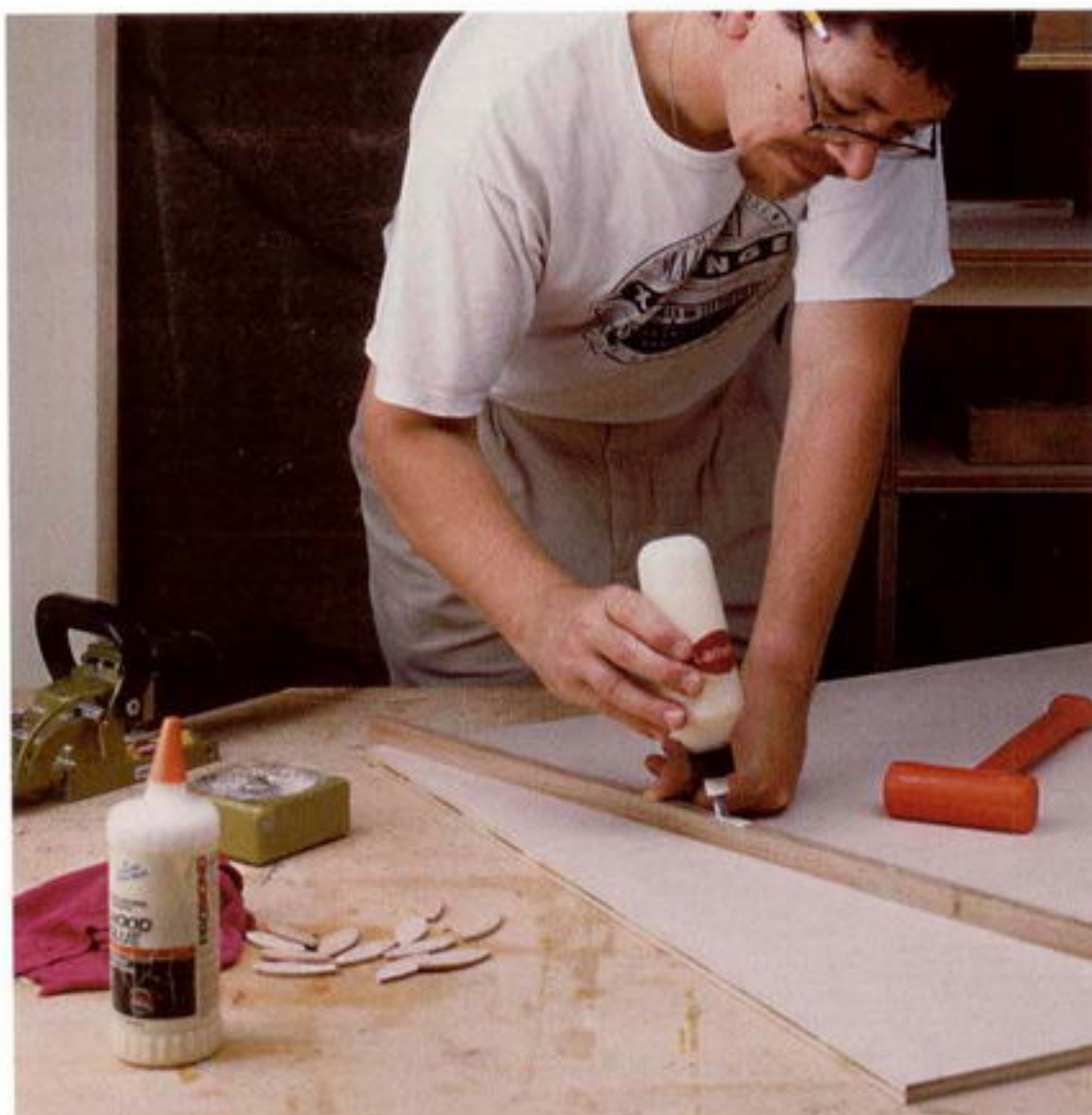
Photo 1: Use biscuits to align the solid butternut strip on the top of the back.
