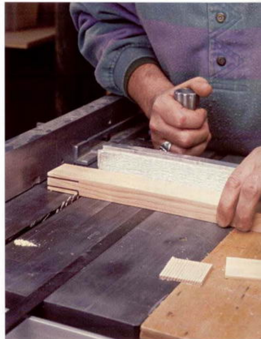
Photo C: The blade should be just high enough to remove the tenon waste when you cut the shoulders.
