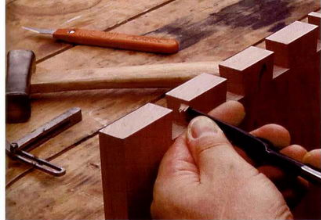
Photo A: Saw, then pare the tails with a chisel until you're satisfied they're right on. You'll use them to mark out the exact locations of the pins on the sides.
