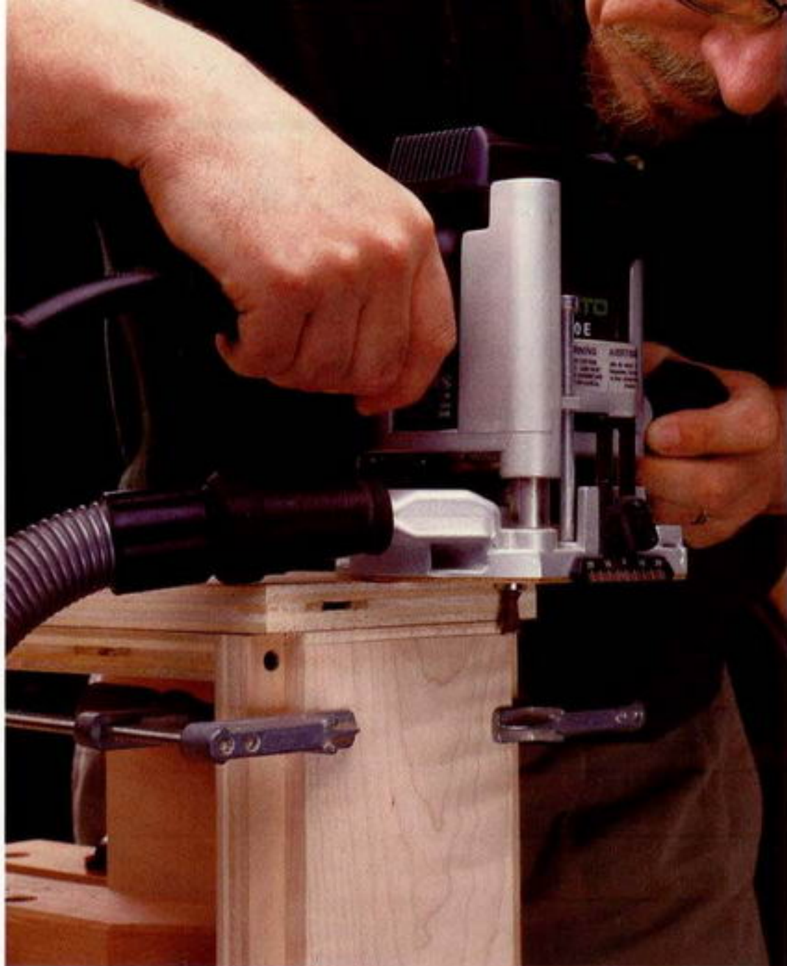
Photo B: The jig for routing tails holds the shelf vertical and cuts one side of the tail at a time. It is accurate, if a little fussy to set up.
