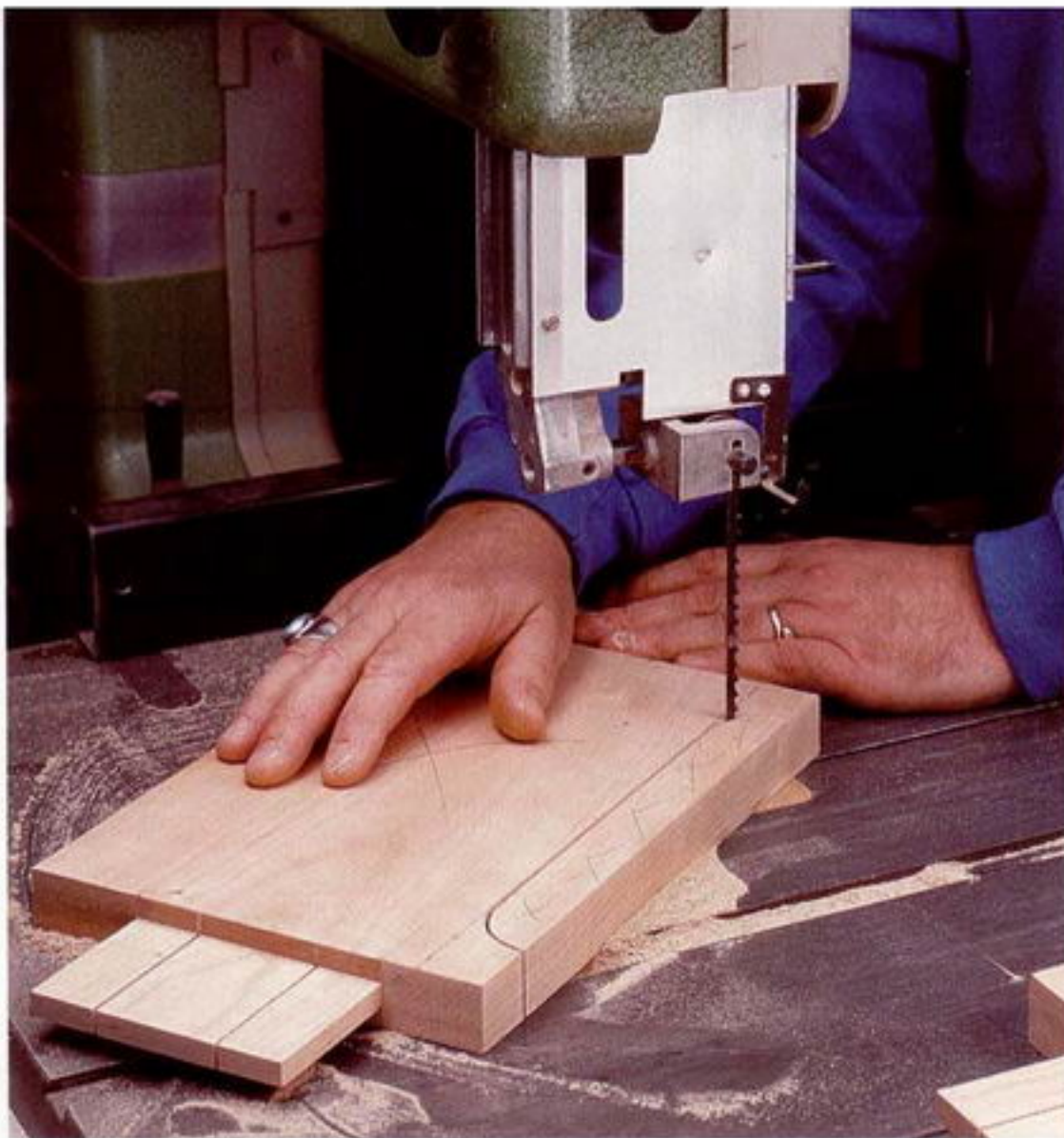
Photo F: A \frac{1}{4} -in.-wide blade on the bandsaw is thin enough to cut out the round corners of the rail details.
