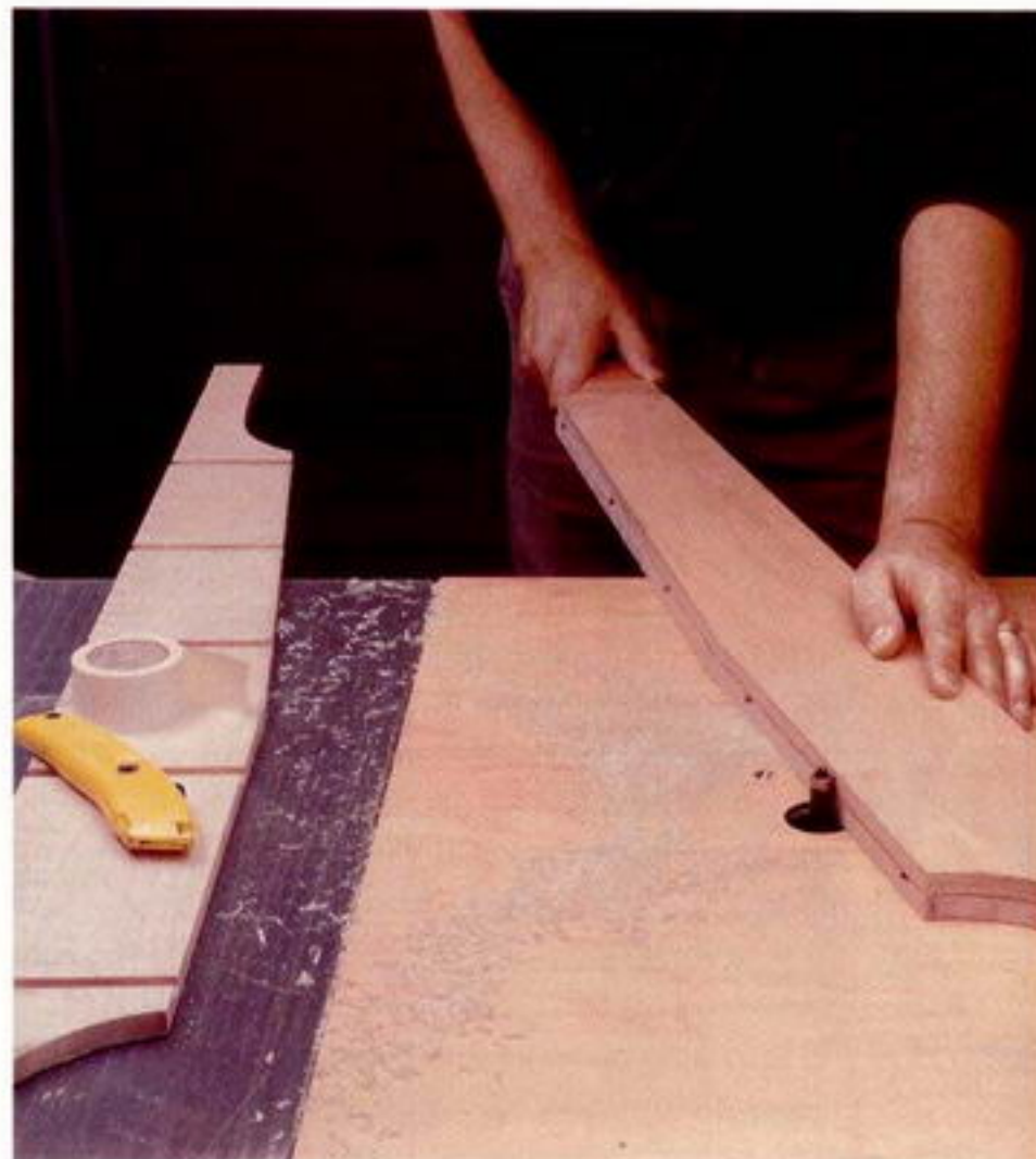
Photo D: The plywood pattern helps you rout a smooth near-perfect edge on the profile of the sides.
