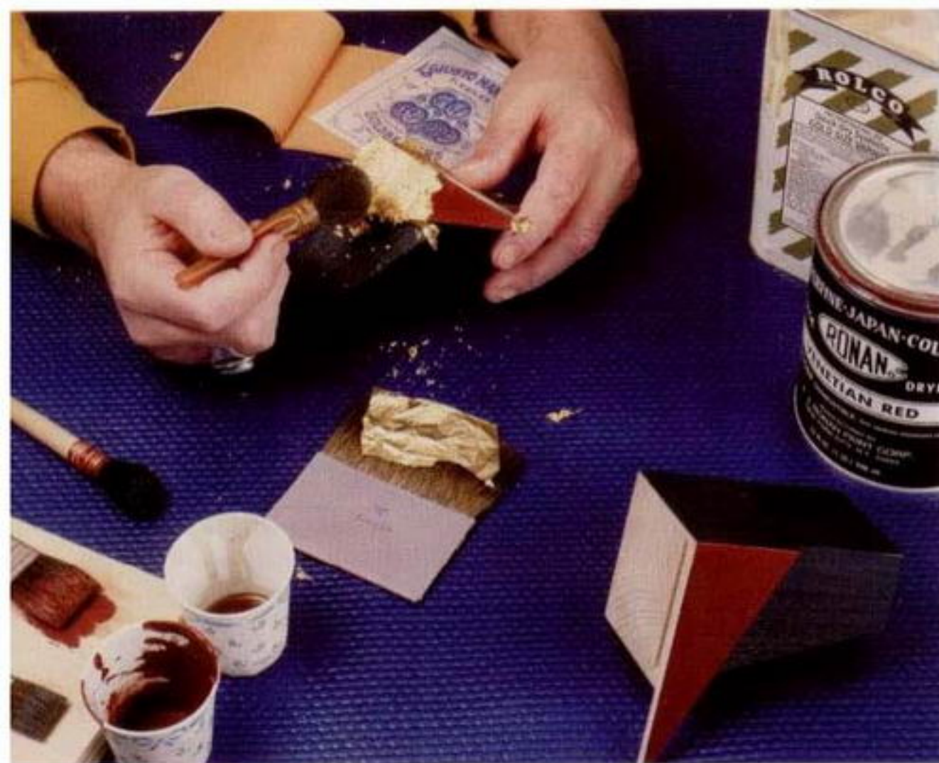
Photo J: Gilding the wings involves the use of several brushes, Japan color, size varnish, and gold leaf. Nevertheless, it is no more difficult than most other finishing processes.
