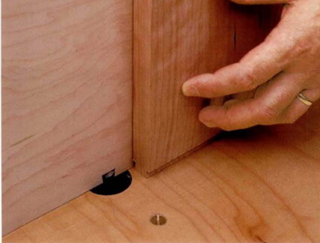
Photo I: A tall fence on the router table guides the shelves when cutting the dovetails on the ends.
