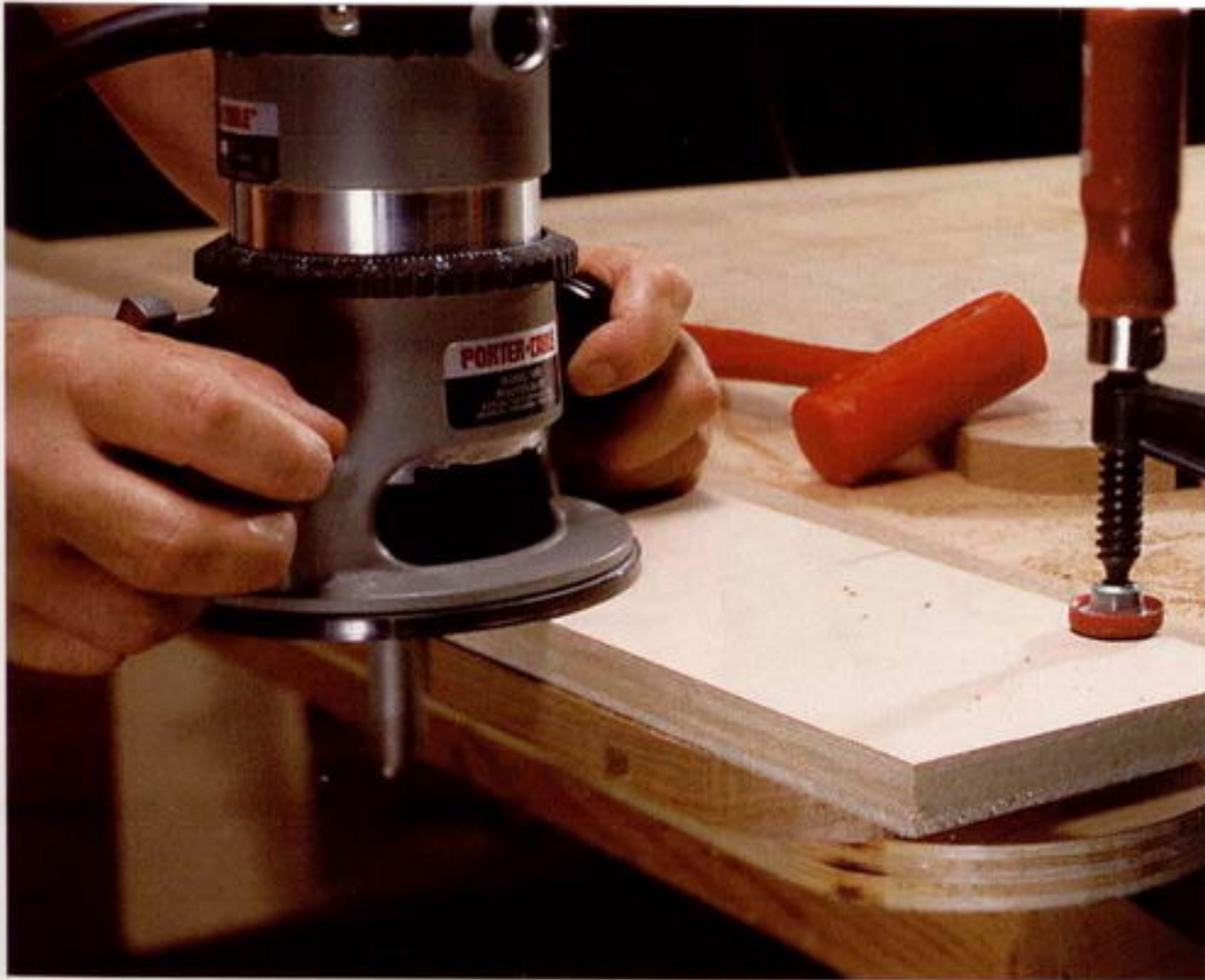
Photo G: With a straight plywood board to guide the router, trim the edge of the case side with a straight bit. Don't worry about smoothing the radius this way. It's best done by hand later.
