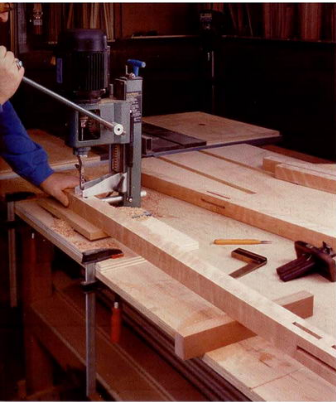
Photo A: A hollow-chisel mortiser cuts square mortises in the posts quickly and efficiently.
