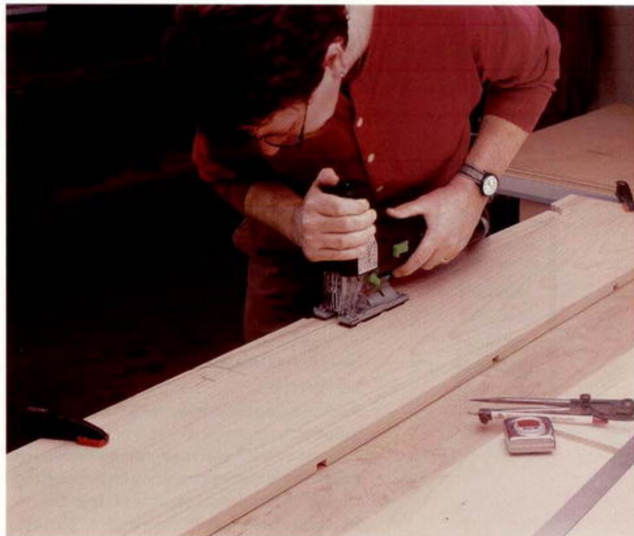
Photo B: Use a jigsaw to cut the profiles in the front edges of the sides. These pieces are too large to cut comfortably on a bandsaw.
