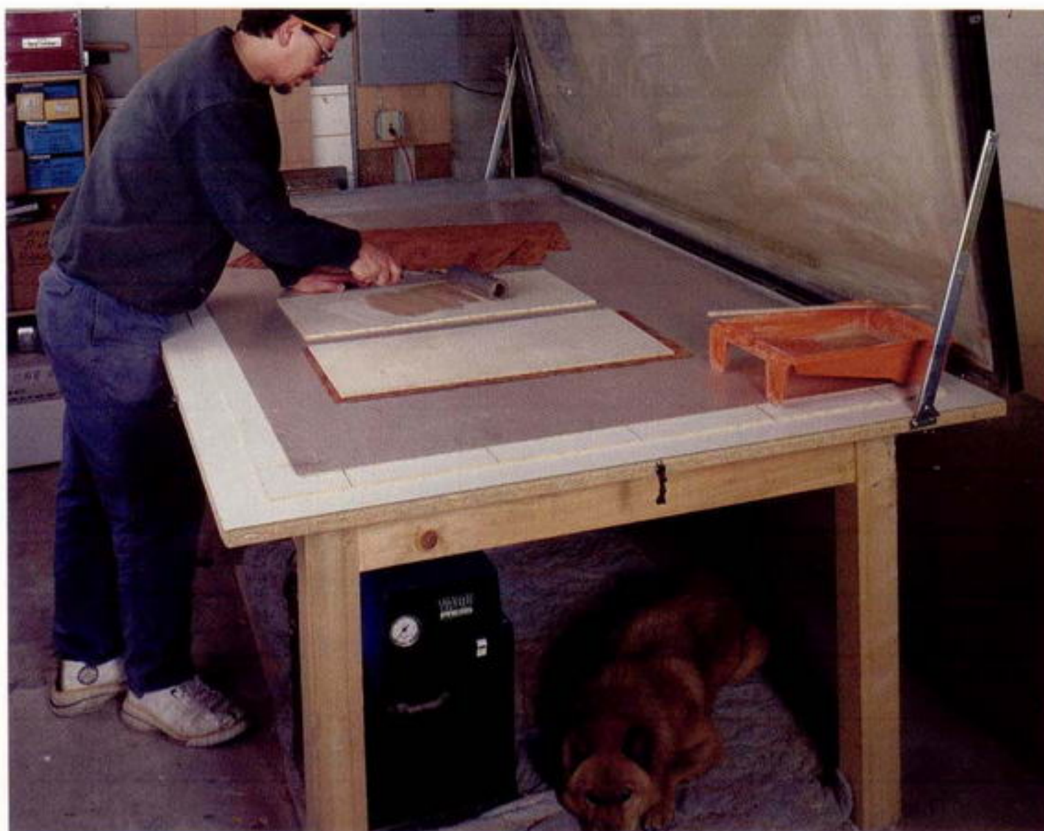
Photo H: Veneer both sides of the door panels and clamp them together in a vacuum or other type of veneer press.
