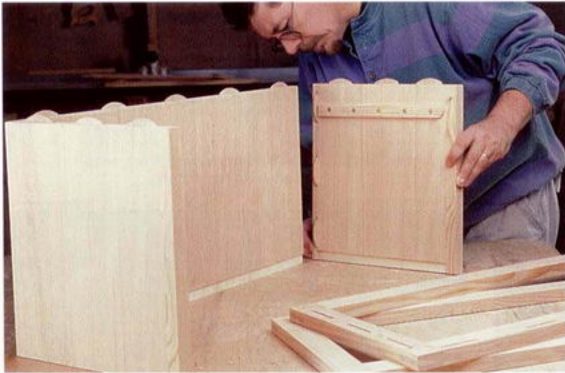
Photo F: Assemble the sides and back of the case before you set them into the frames because it's not possible to do it any other way.
