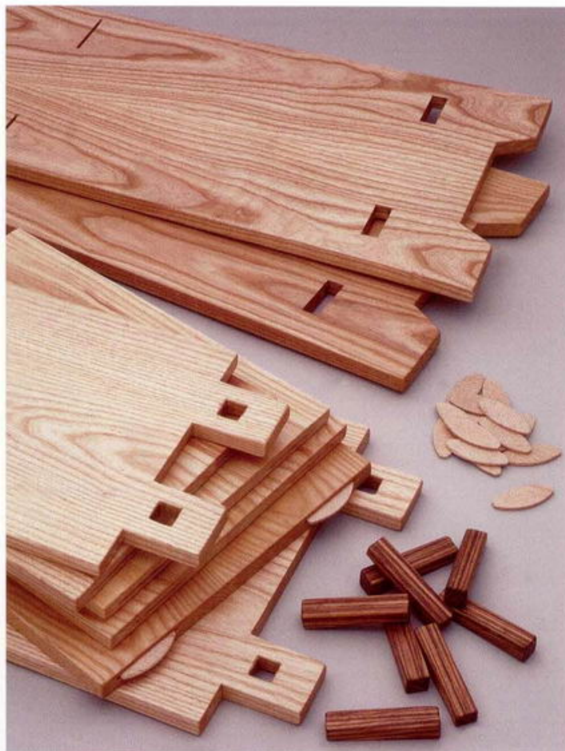
Photo K: The entire bookcase knocks down into a small pile of flat, small pieces—very handy for transportation.
