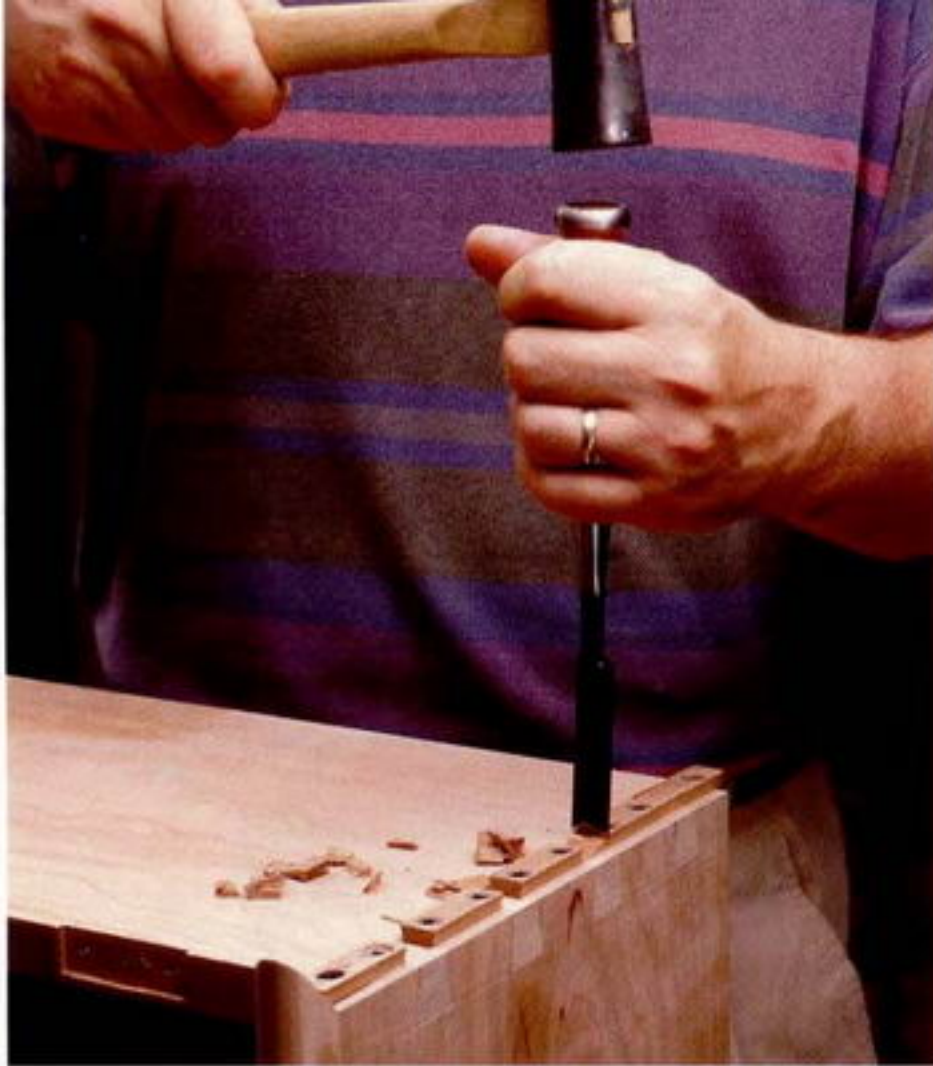
Photo N: Chop out the waste between the keys, don't saw it. A saw might cut into the face or edge of the carcass.
