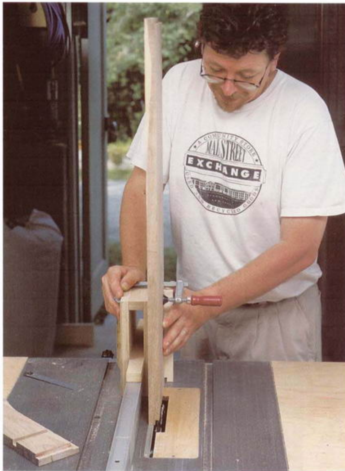
Photo D: A simple shopmade carrier will guide the shelf ends over the dado blade to tenon the ends.
