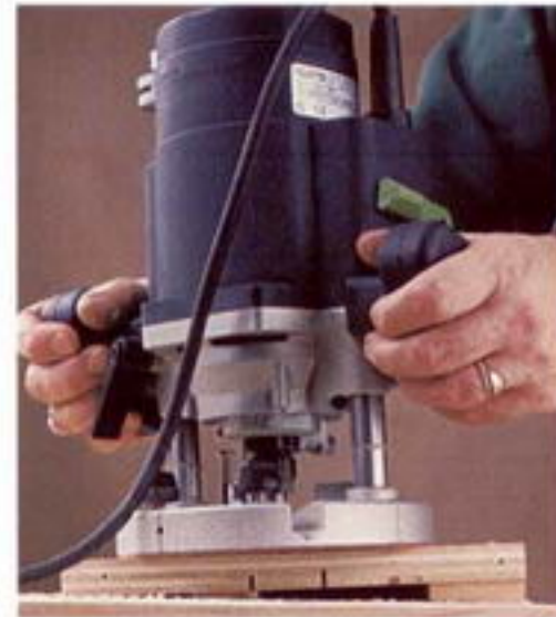
Photo D: The mortising jig tilts the router 3 degrees and cuts the mortise walls at the same angle.
