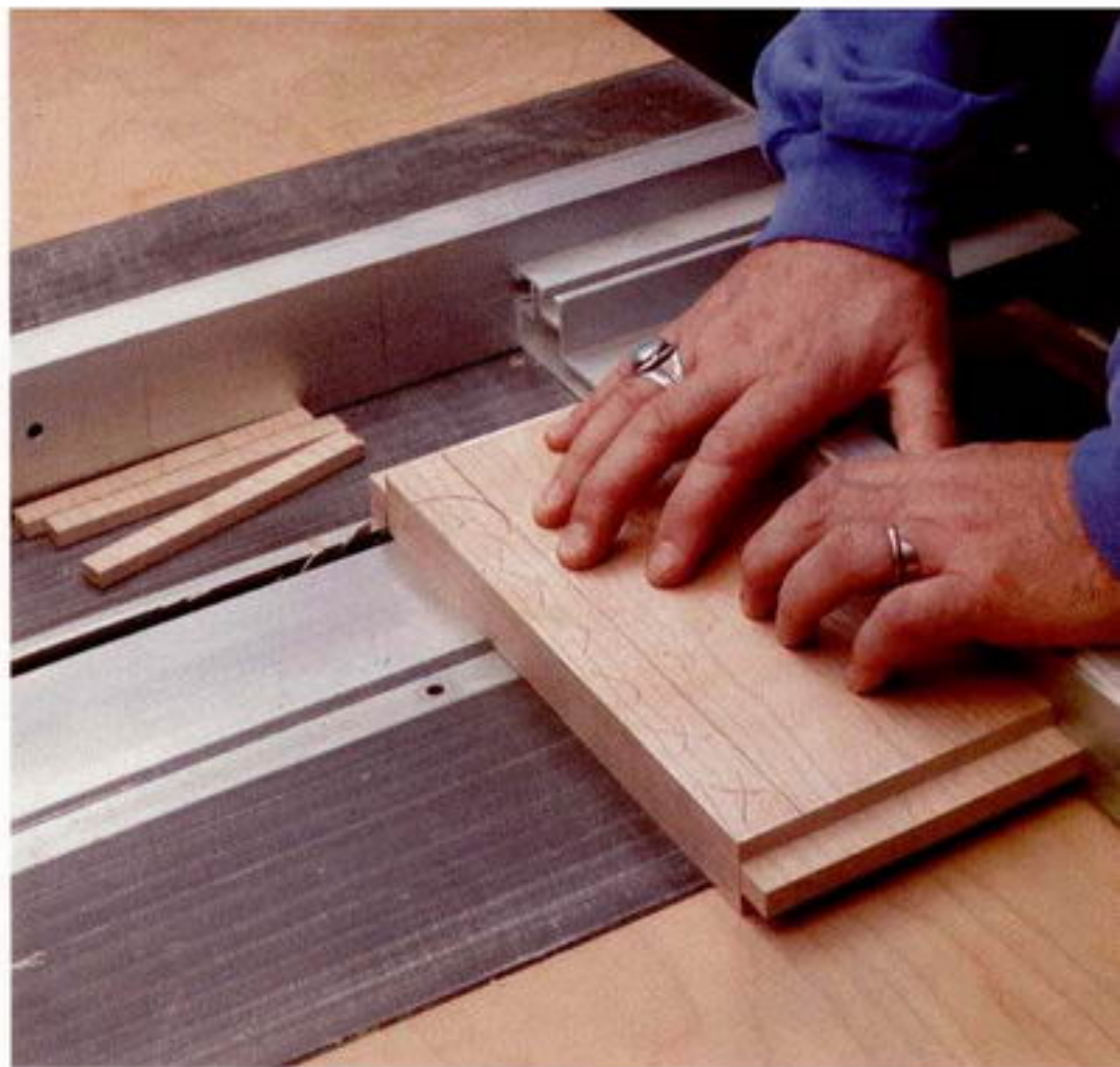
Photo E: Cut the tenon shoulders on the table saw for a clean edge.
