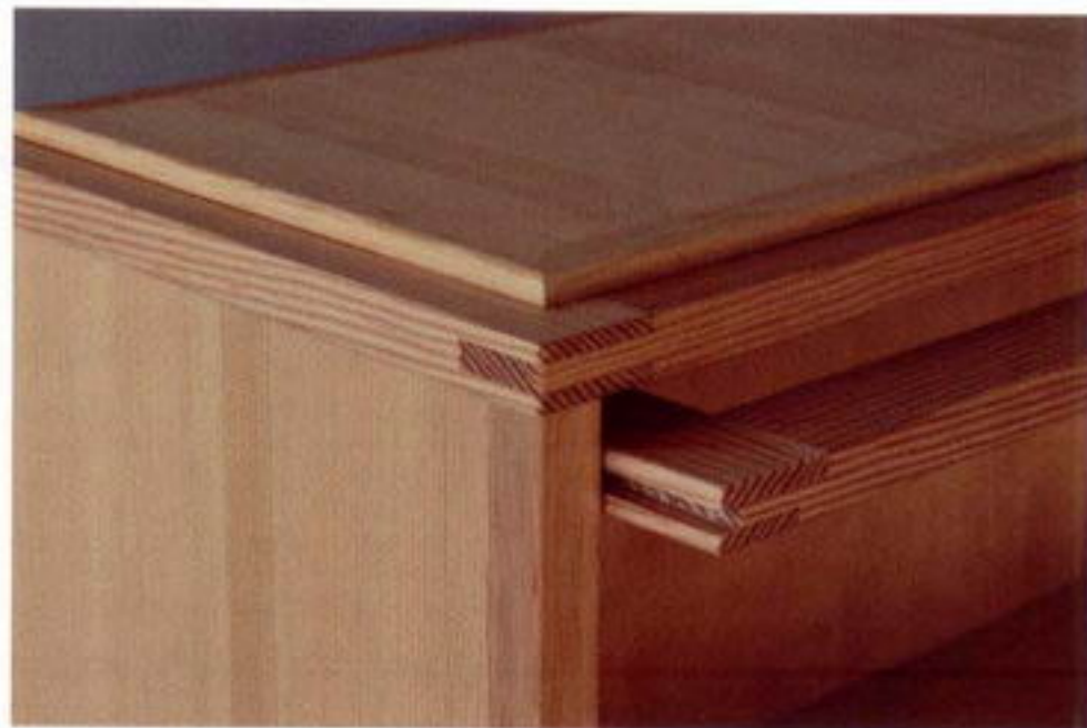
When open, the door reveals the groove in the edge that rides on the pin in the case.
