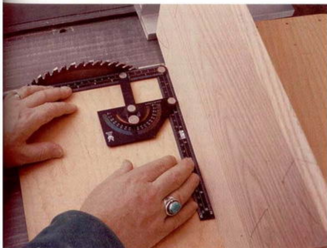
Photo G: To cut the outside tenon shoulders, reposition the box fence 3 degrees to the blade.
