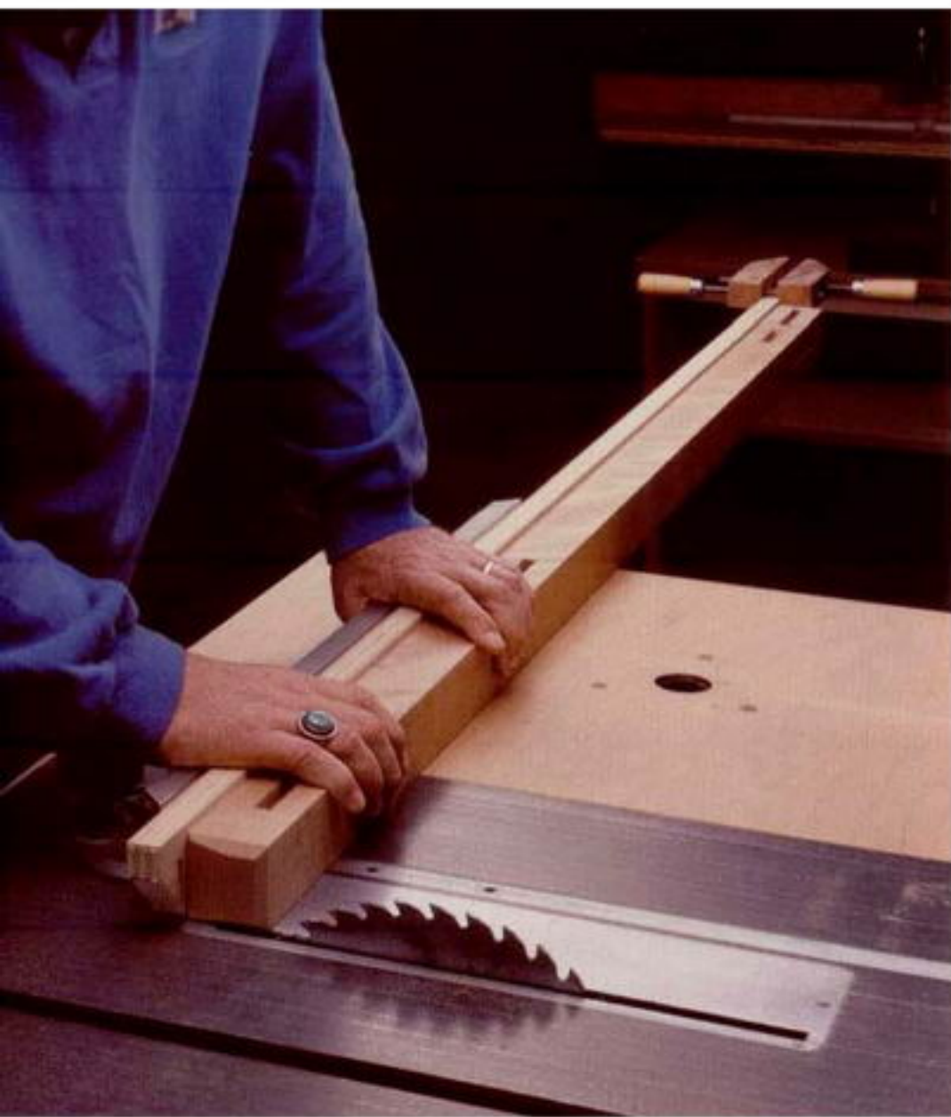
Photo C: Cut the two bevels on the top of the posts on the table saw with a miter gauge.
