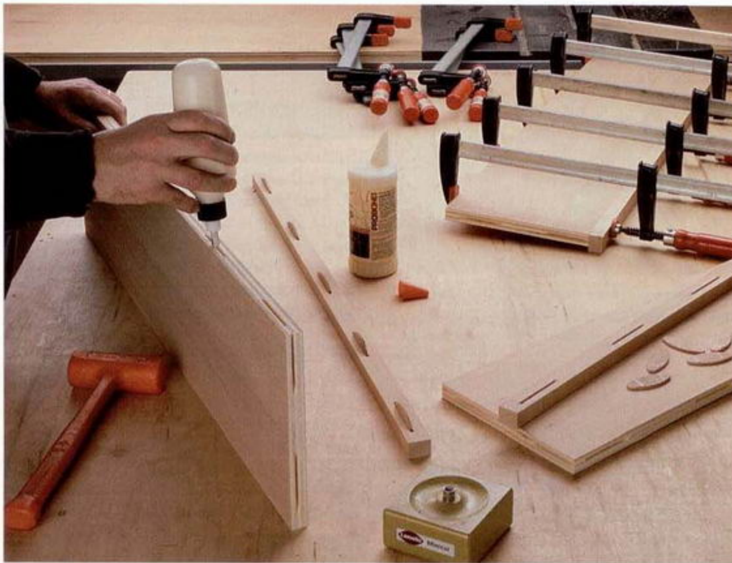
Photo A: Solid-wood edging is attached to the front edges of the plywood shelves.
