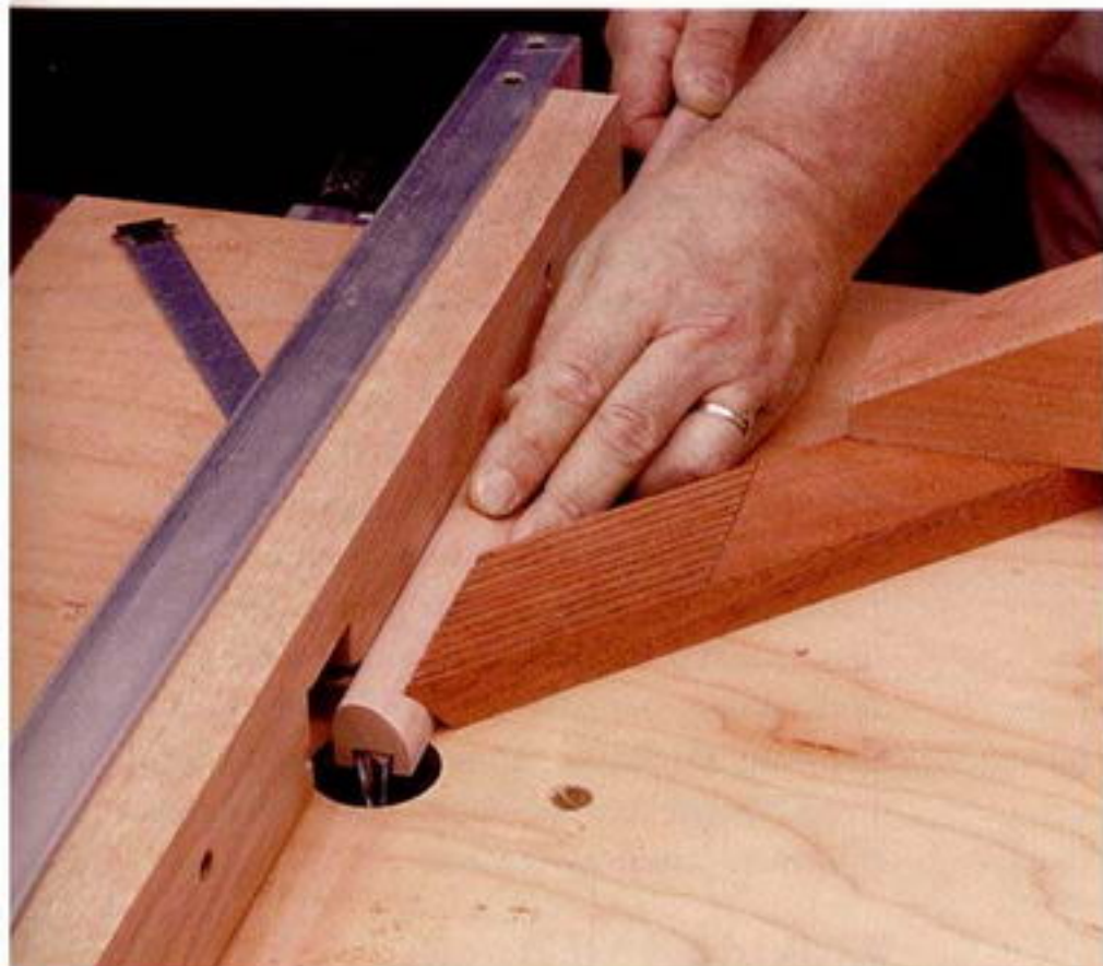
Photo L: Rout the dovetail slots in the molding on the router table. Use an angled featherboard to keep the molding against the fence. Apply solid downward pressure when routing the slots. Any unwanted movement of molding will ruin the slots.
