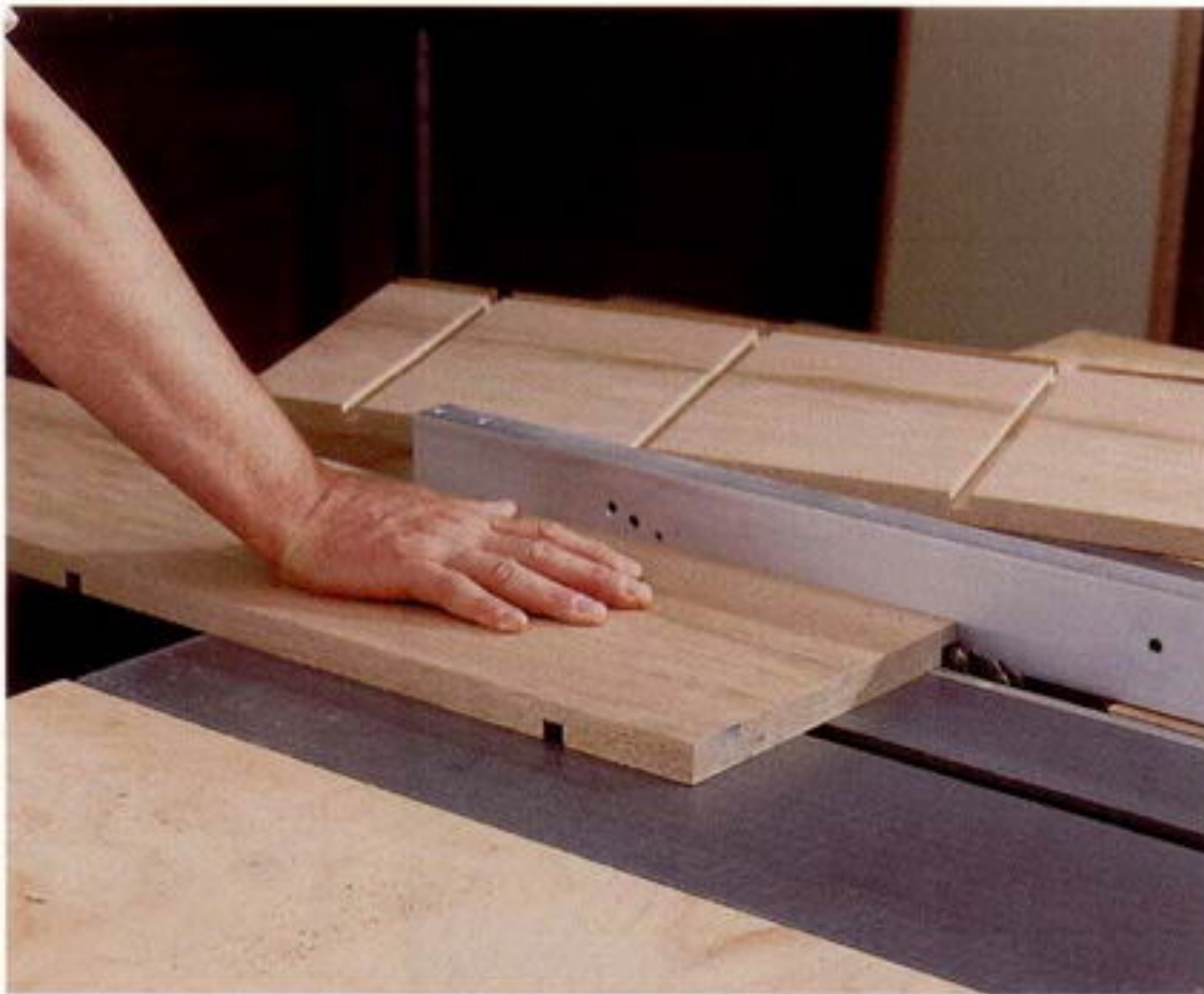
Photo C: The same dado blade at the same height setting will cut the rabbets for the back.
