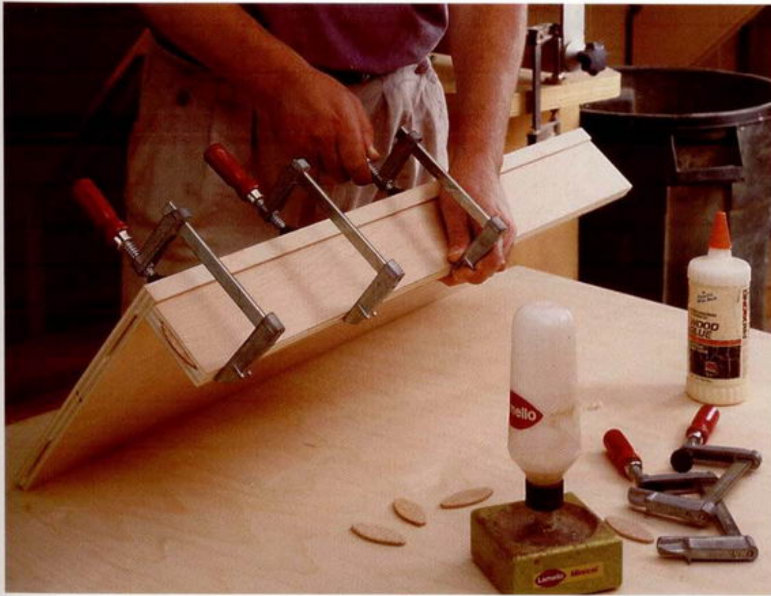
Photo G: Assemble the bottom shelf and kick board before you glue up the entire case. This will make the overall glue-up less complicated.
