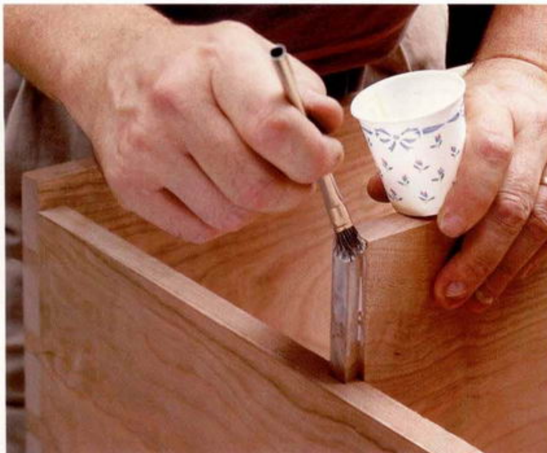
Photo J: Apply glue to the shelf dovetails only after they're most of the way into their slots. Also, spread some glue in the slots at the back of the shelves.
