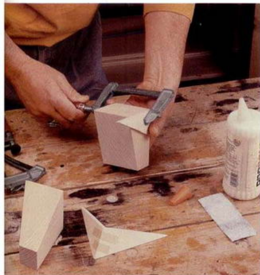
Photo 1: Tape, clamps, and glue are all you need to join the wings and attach them to the feet, flush with the top.
