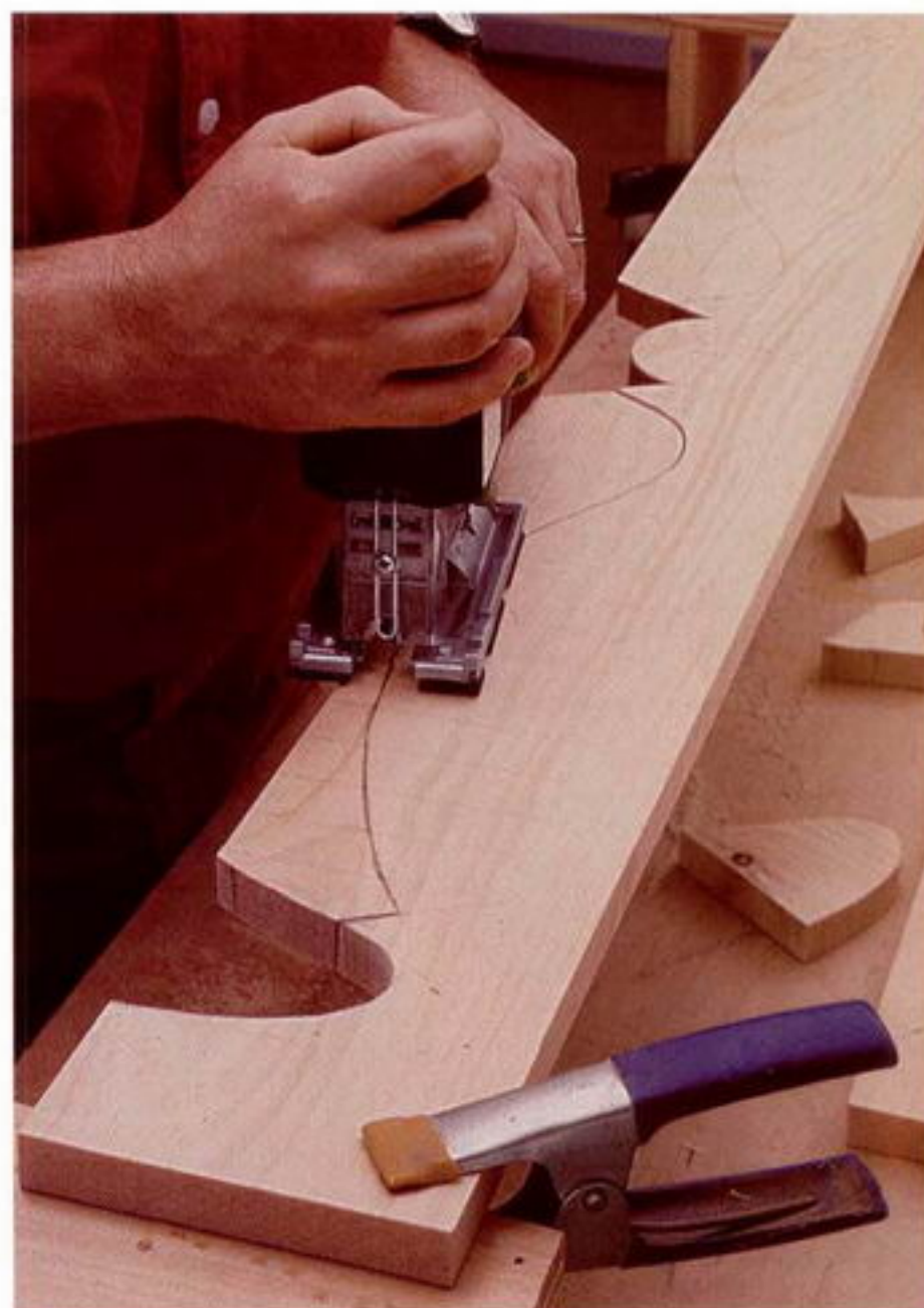
Photo E: A jigsaw with a fine blade will cut the profiles cleanly.
