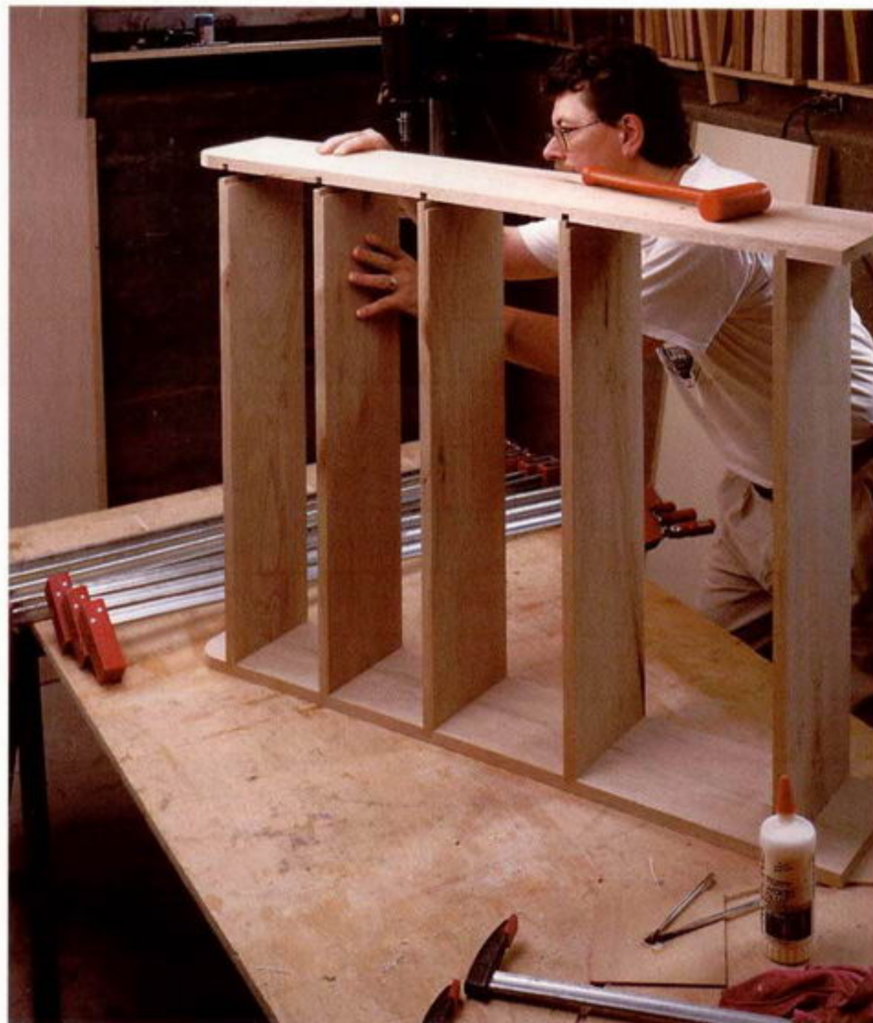
Photo K: Glue-up can be a hectic time, so make sure you have all the clamps and pieces ready to go and proceed in a quick but orderly fashion.
