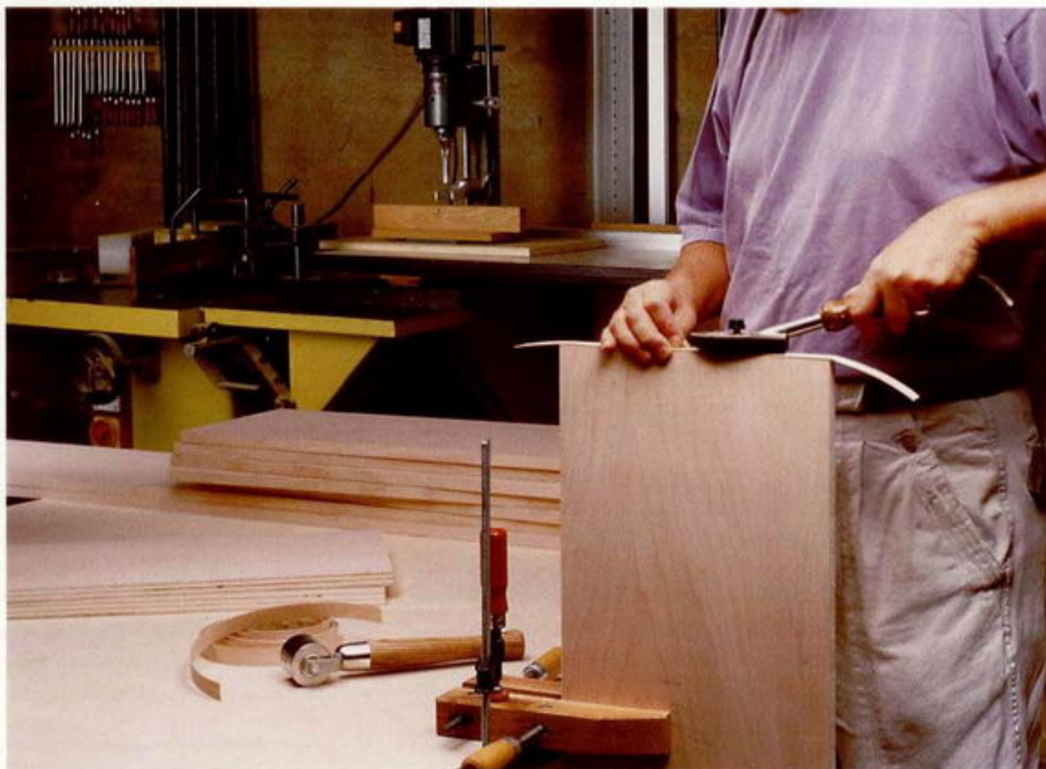
Photo F: With an edge-banding iron, I apply banding to all edges that show.
