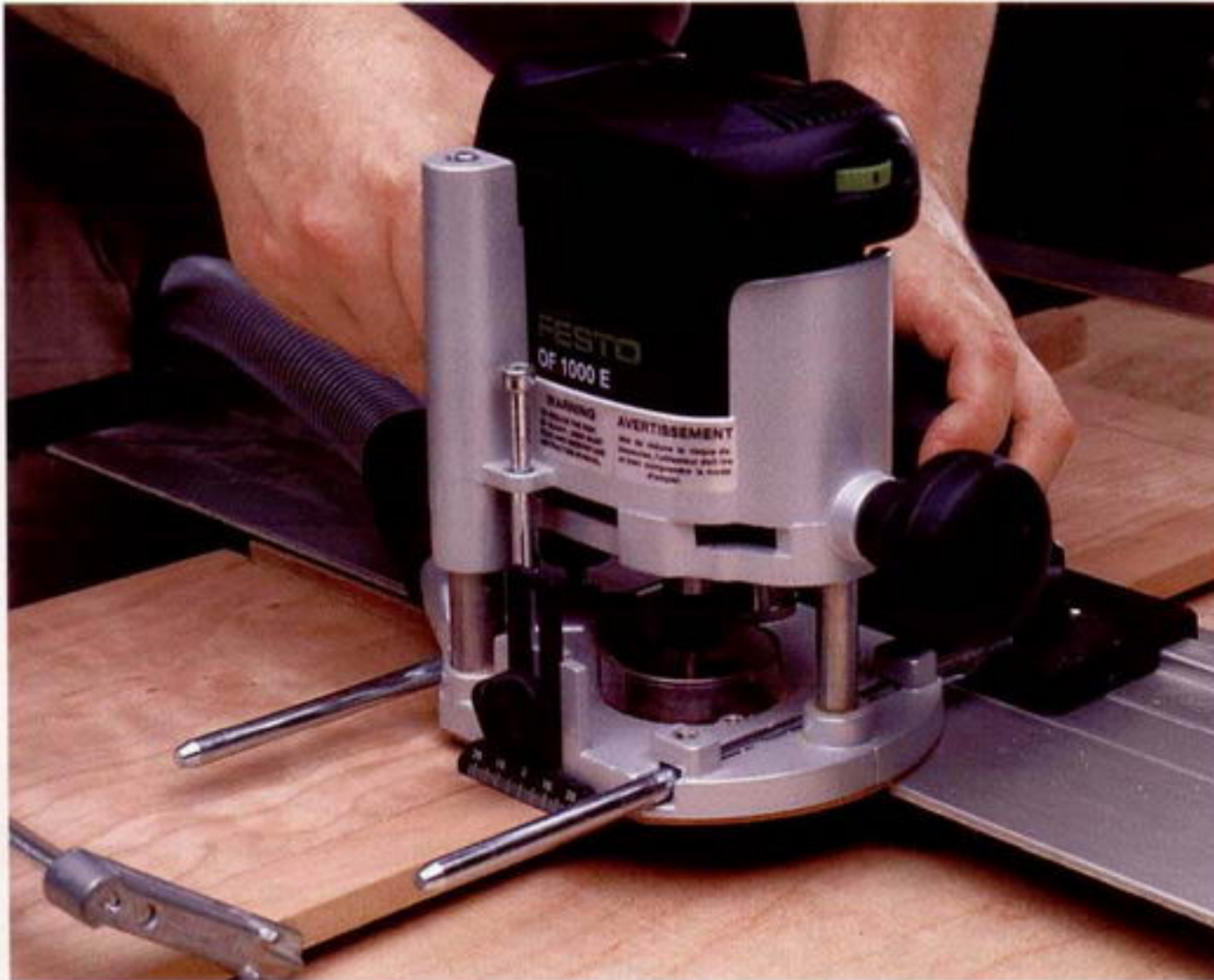
Photo G: Routing the dovetail slots is simple with a guide rail fixture. This Festo guide rail clamps to the board at 90 degrees and guides the router through the cut. With a piece of scrap clamped at the end, the bit won't splinter the grain where it shows.
