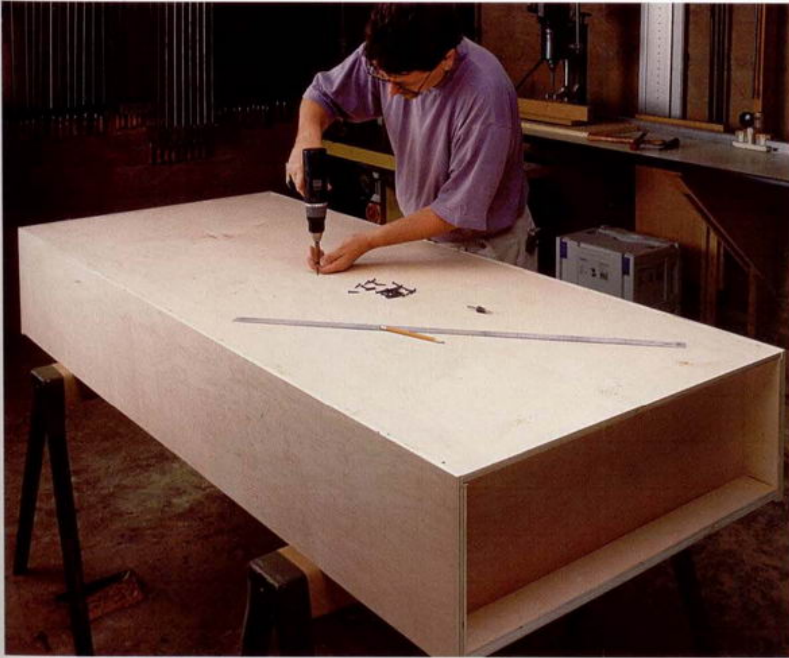
Photo 1: Screw on the back with trim-head screws. These have very small heads that make them ideal for attaching the back along the thin rabbeted edge.
