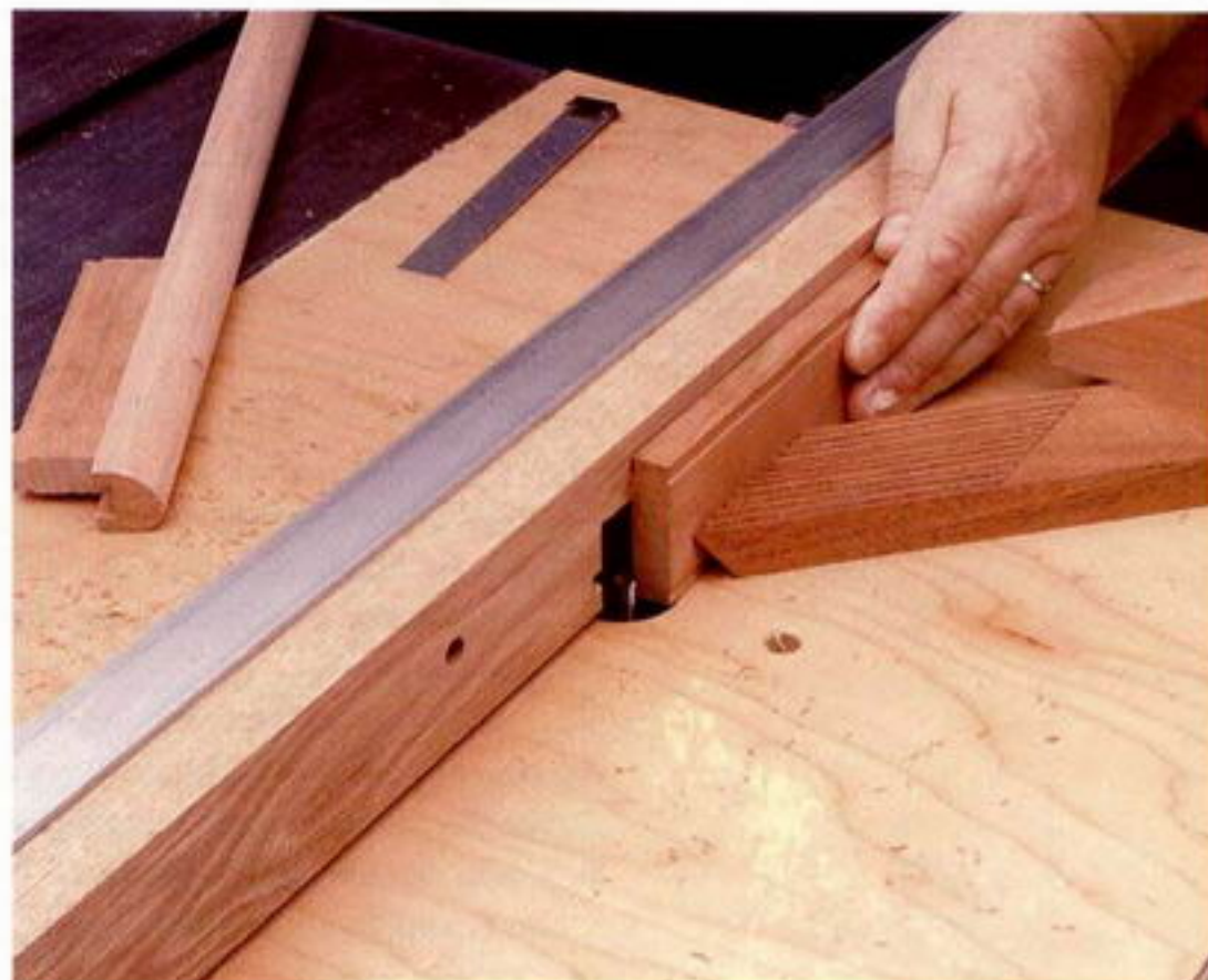
Photo M: To make the dovetailed keys, first make some test pieces and fit them to the molding. Then run the key stock through on both sides.
