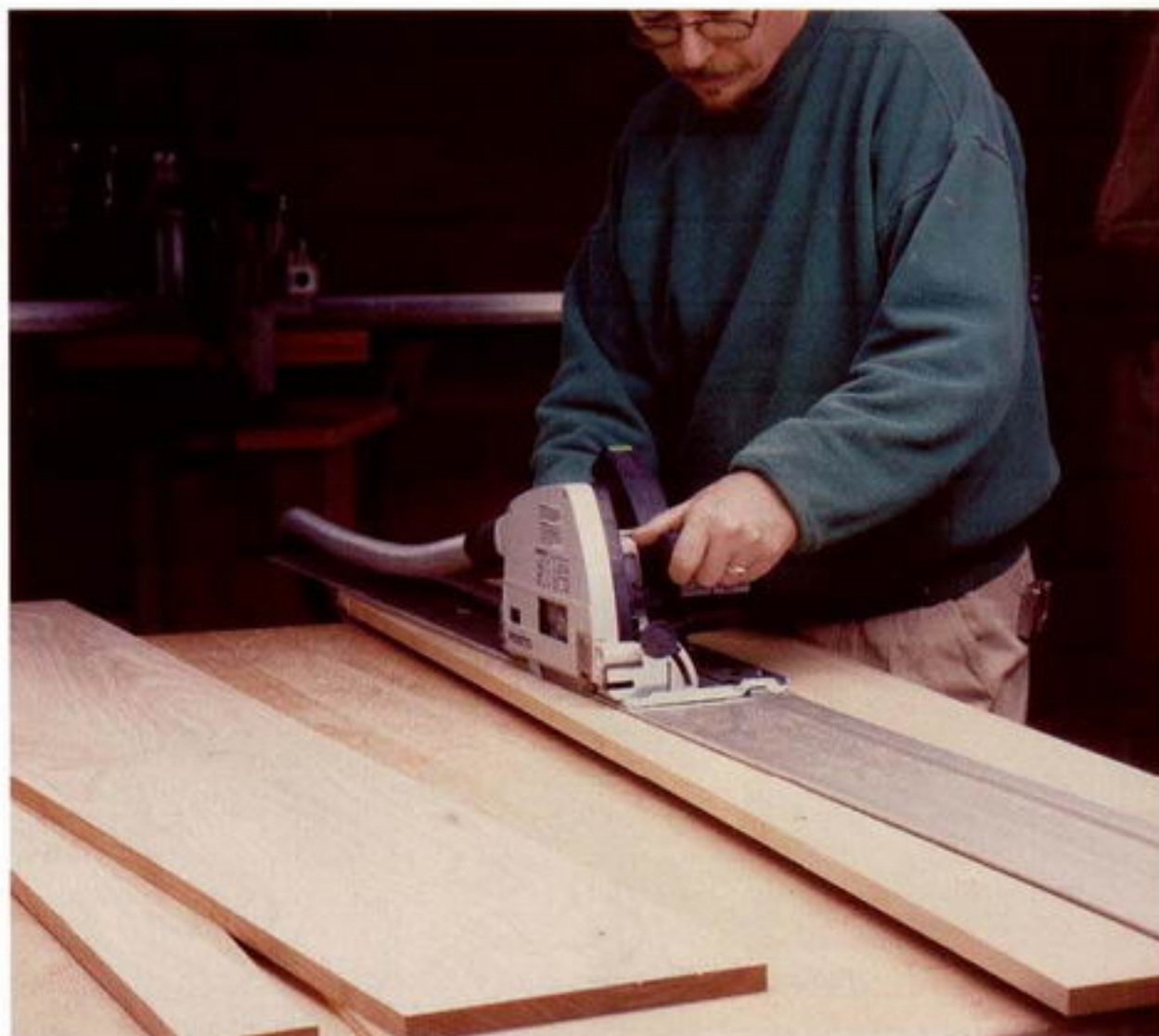
Photo B: A circular saw and straightedge guide make cutting the tapers on the sides a cinch.
