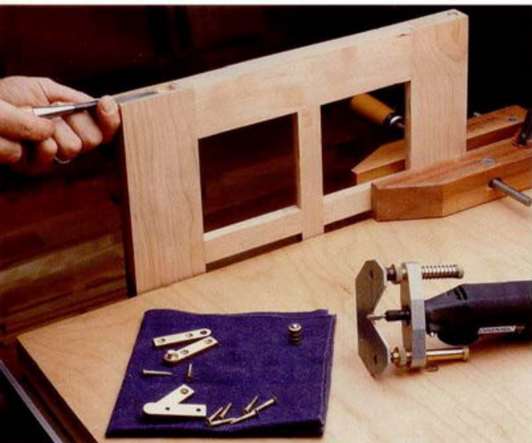
Photo I: Rout the waste out of the knife-hinge mortise, and clean up the edges with a chisel.
