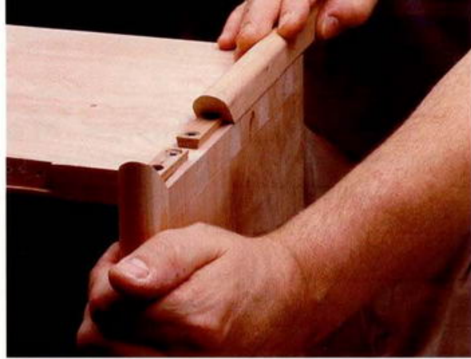
Photo O: The thumbnail molding shouldn't slide on too easily but shouldn't need to be hammered into place.
