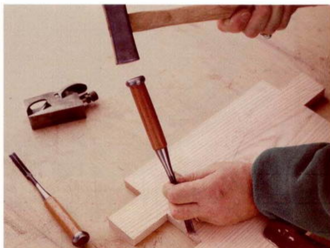
Photo H: Clean up the jigsaw cut with a chisel.
